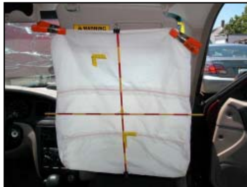
Figure 11. Deployed front right passenger's air bag
