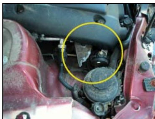
Figure 6. Close-up of fractured motor mount
