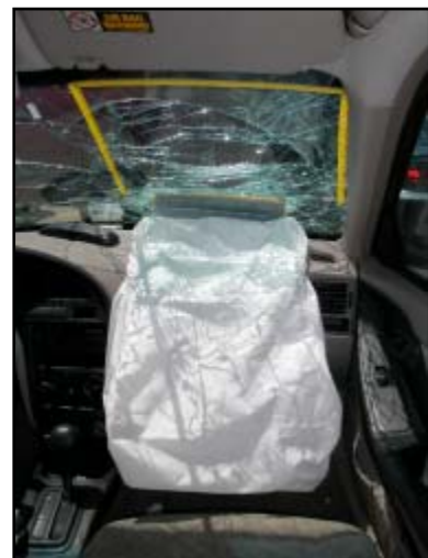
Figure 10. View of cover flap, fractured windshield, and transfer area
