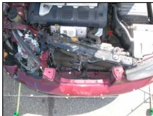
Figure 5. Overhead image of the frontal damage to the Elantra
