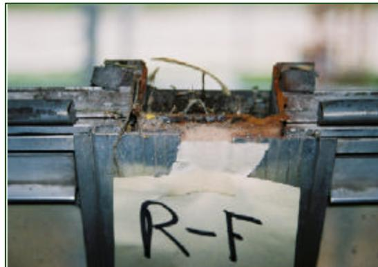
**Figure 12.** Separation of the right F-pillar.
