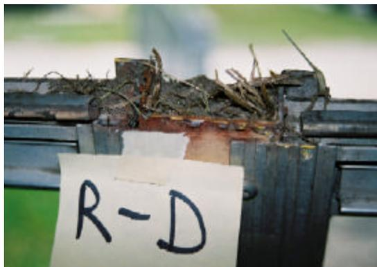
**Figure 11.** Separation of the right D-pillar.
