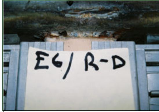
**Figure 25.** Crack side and face welds of right D-pillar of Exemplar Bus No. 6.
