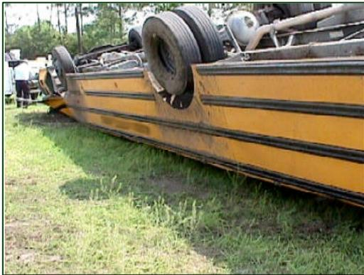
**Figure 7.** On-scene image of the roof collapse at the right side.
