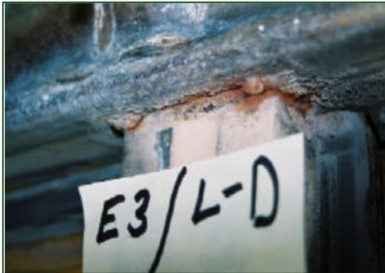
**Figure 18.** Cracked weld at the left D-pillar of Exemplar Bus No. 3.
