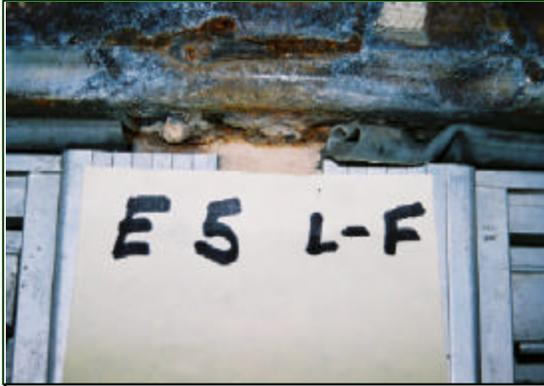
**Figure 22.** Cracked weld at left F-pillar of Exemplar Bus No. 5.
