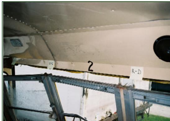
**Figure 6.** Separation of the right A- through I-pillars.
