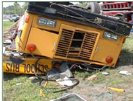
**Figure 2.** Collapsed roof of the 1991 Carpenter school bus.
