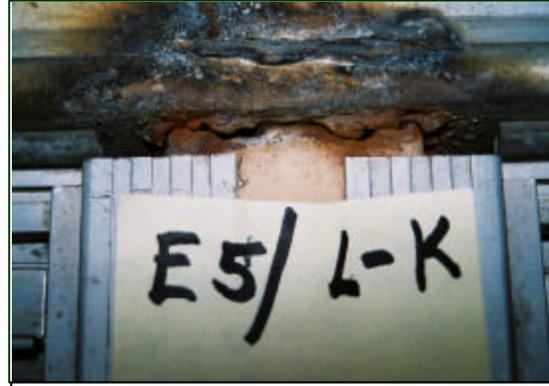
**Figure 23.** Complete crack of weld at left K-pillar of Exemplar Bus No. 5.
