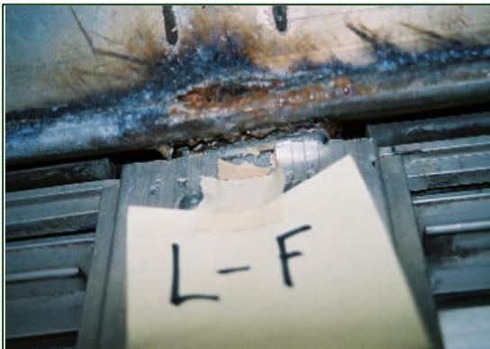
**Figure 9.** Crack at left F-pillar weld.
