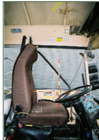
**Figure 14.** Driver’s seat and contact points.
