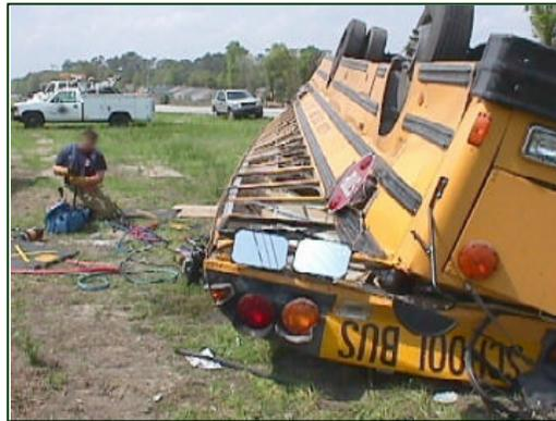
**Figure 8.** Left side roof collapse as viewed from the front of the Carpenter school bus.
