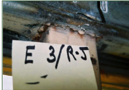
**Figure 19.** Cracked weld at the right J-pillar of Exemplar Bus No. 3.
