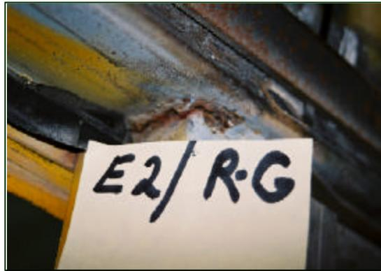
**Figure 17.** Cracked weld at the right G-pillar of Exemplar Bus No. 2.
