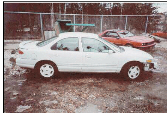
Figure 5: Right side of case vehicle at tow yard; note front right corner of bumper cover broken away (case photo #21)
