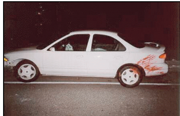
Figure 4: Left side of case vehicle on-scene; note, left bumper cover broken away, left front wheel displaced rearward, blood from moose on left rear quarter panel (case photo #09)
