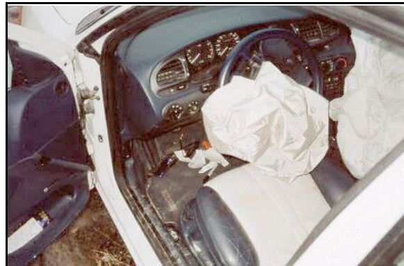
Figure 6: Case vehicle's front seat, showing deployed air bags (case photo #24)
