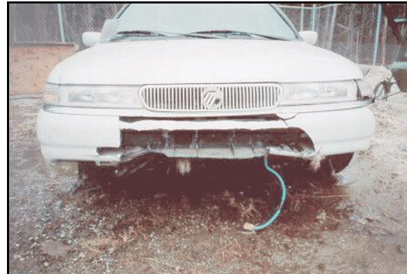
Figure 3: Front of case vehicle at tow yard; note tufts of moose fur (case photo #13)
