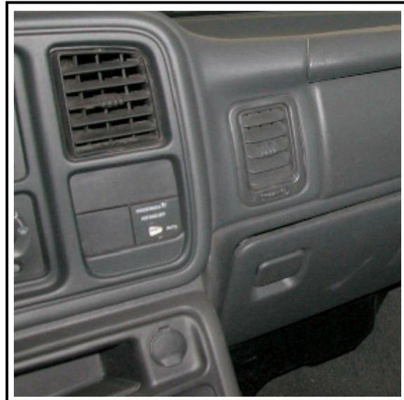
**Figure 11.** Passenger air bag cut off switch in AUTO position
