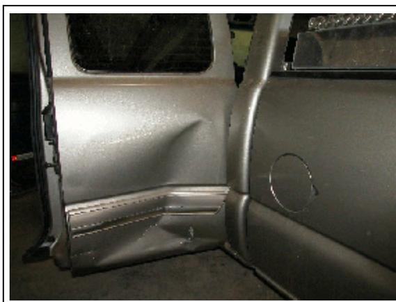
Figure 5. Side slap damage to left rear door panel
