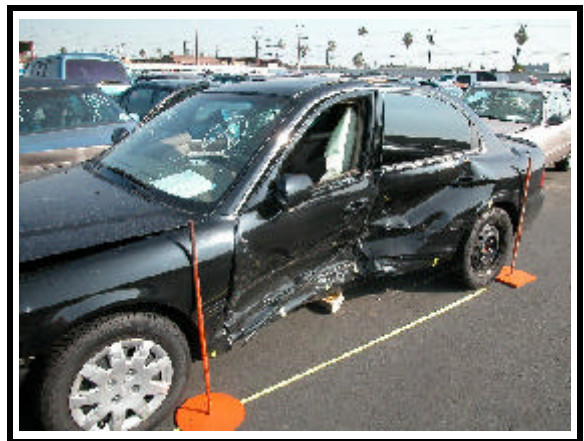
Figure 3. Left side damage (impact 1) to case vehicle.
