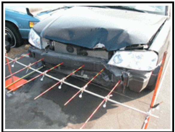
Figure 4. Front damage to case vehicle (impact 2).
