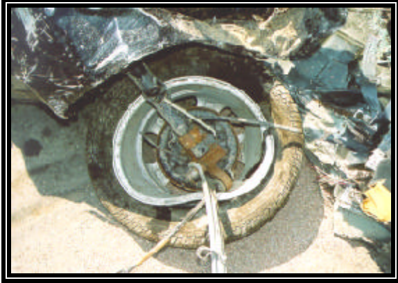
Figure 7: Right rear wheel impact damage.
