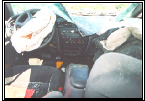
Figure 9: Front interior view and center console deformation.
