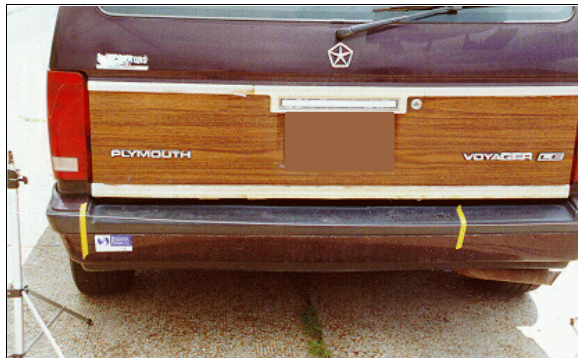
Figure 4: Contact (taped) on Plymouth's bumper showing minimal deformation (case photo #41)
