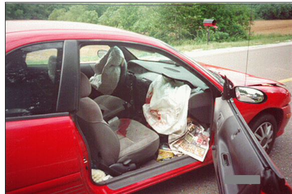
Figure 5: On-scene view of case vehicle's front right seating area showing excessive blood on seat and deployed passenger air bag; Note: front right seat track was moved backward by rescue personnel (case photo #49)
