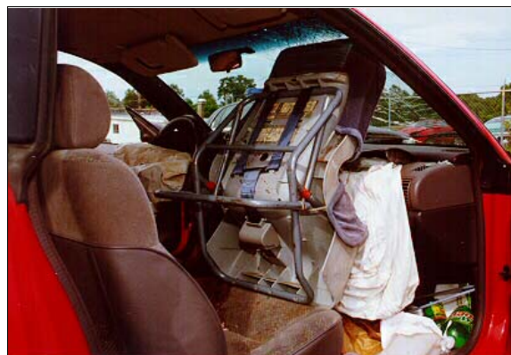
Figure 23: Case vehicle's front right seating area showing approximation of position of unsecured forward facing child safety seat at deployment (case photo #36)
