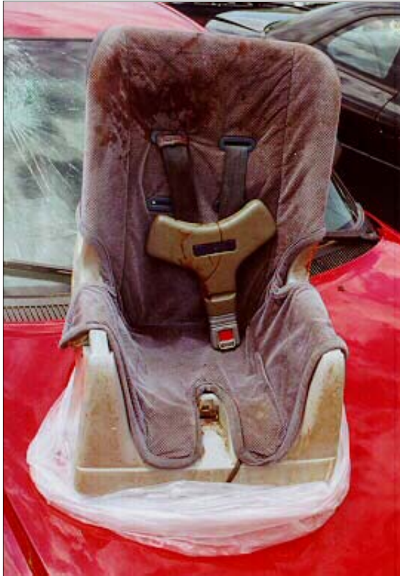
Figure 18: Frontal view of bloodied Fischer/Price model 9100 convertible child safety seat used by case vehicle's front right passenger (case photo #37)
