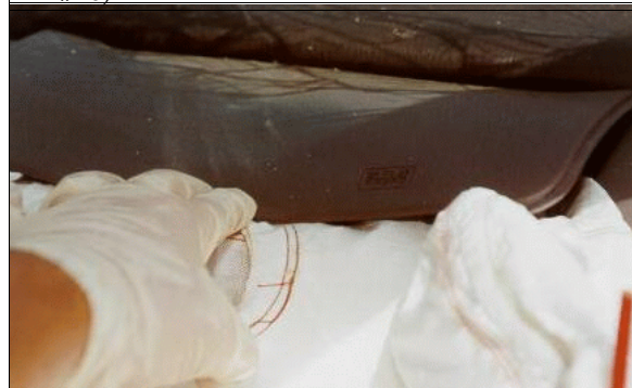
Figure 16: Deformation and contact evidence on cover flap of case vehicle's front right air bag module (case photo #32)
