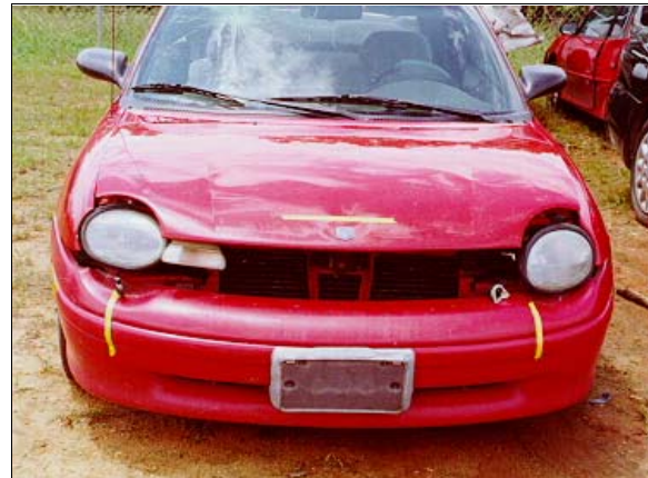
Figure 3 Case vehicle's minor frontal damage from underride impact; Note: tape indicates area of direct contact (case photo #05)
