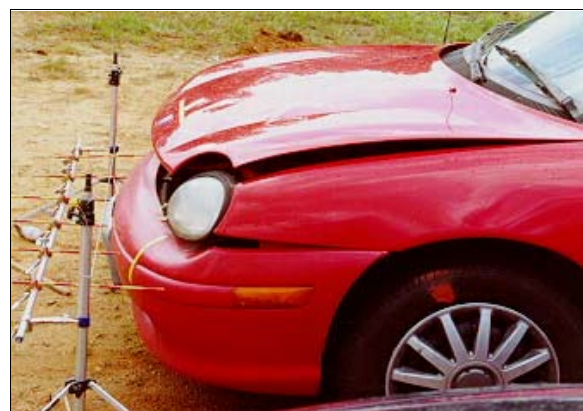
Figure 6: Reference line view from left showing case vehicle's front deformation; Note: damage primarily above bumper (case photo #09)
