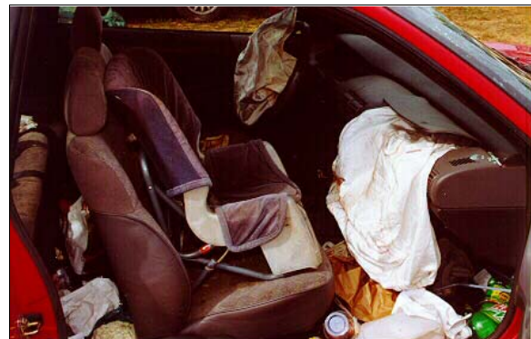
Figure 22: Case vehicle's front seating area showing deployed air bags and unsecured forward facing child safety seat in its pre-impact position (case photo #22)
