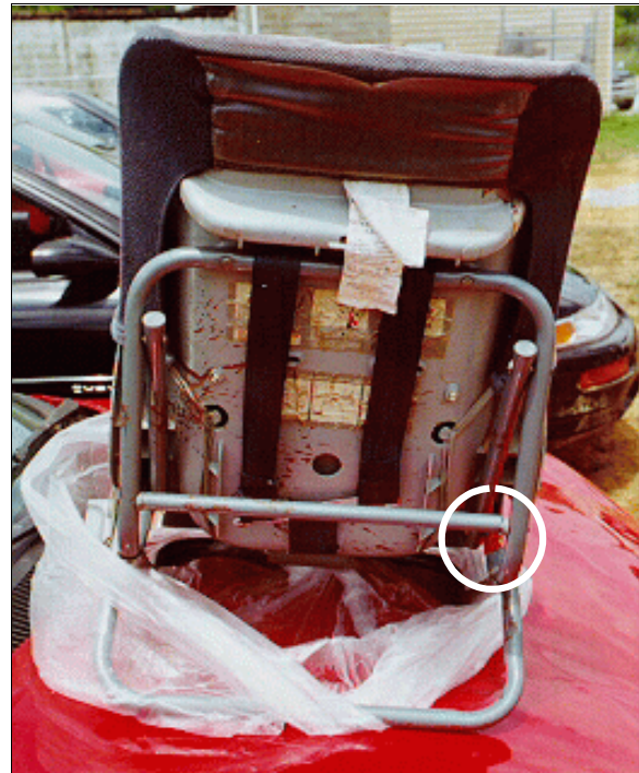
Figure 20: Back view of Fischer/Price model 9100 used by case vehicle's front right passenger showing blood splatters and highlighted area of brace displacement (case photo #35)
