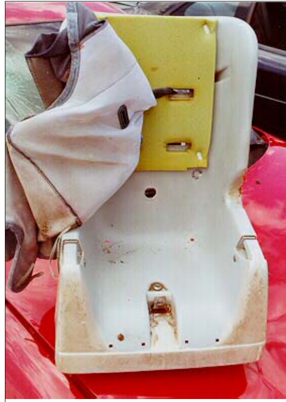
Figure 19: Fischer/Price model 9100 child safety seat used by case vehicle's front right passenger with bloodied cover pulled away showing no visible stress to plastic shell (case photo #37a)
