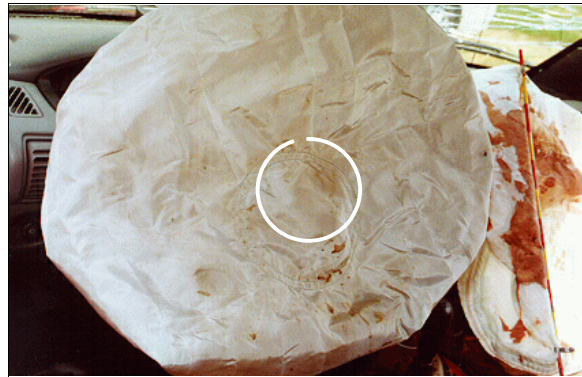
Figure 15: Case vehicle's deployed driver air bag with contact evidence highlighted (case photo #20)
