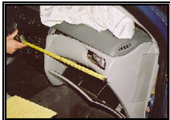
Figure 5: View of the deformed mid panel below the passenger air bag module.
