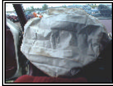
Figure 10. Deployed non-tethered driver air bag.
