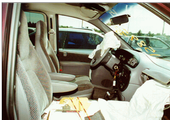
Figure 25: Case vehicle's front seating area showing deployed driver and front right passenger air bags, front bucket seats, and driver's adjustable upper seat belt anchorage, positioned in its down most position
