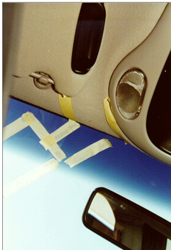
Figure 17: Close-up of contact evidence on case vehicle’s front left header and windshield (i.e., smudging) from impact by “on-lap” infant, front left passenger
