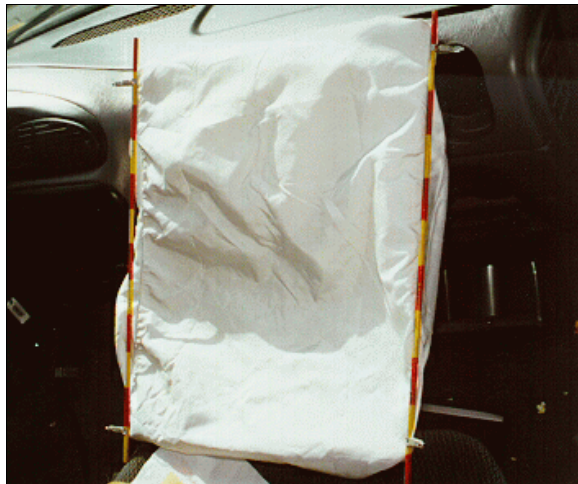
Figure 23: Case vehicle's deployed front right passenger air bag showing no evidence of occupant contact
