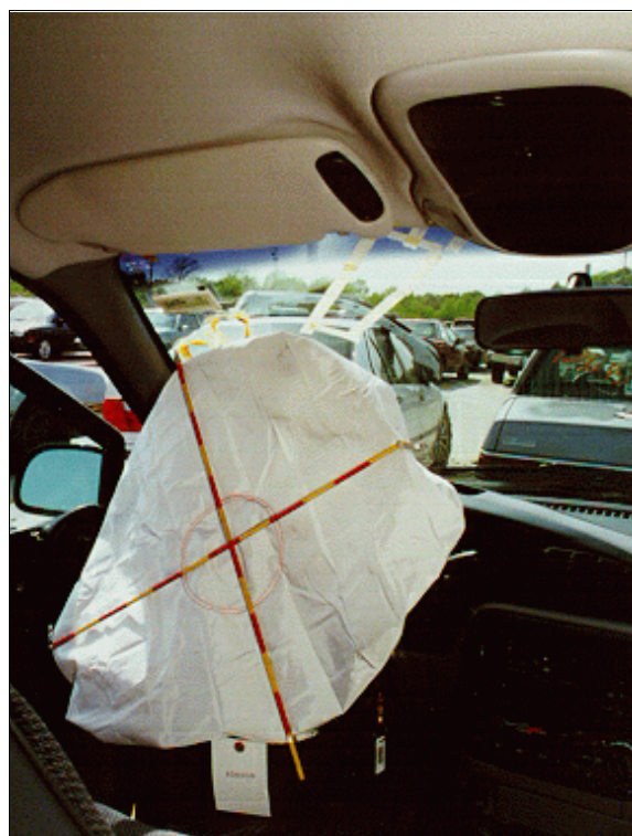
Figure 16: Vertical view of case vehicle's driver seating area showing contacts to front left header and windshield from impact by "out-of-position" (i.e., standing on driver's lap) front left infant passenger
