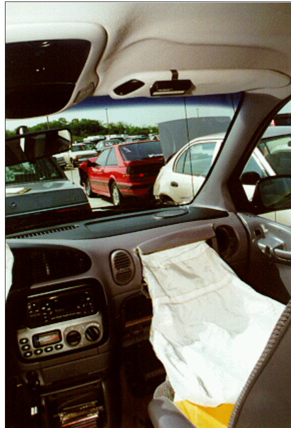
Figure 22: Vertical view of case vehicle's front right seating position showing front right passenger air bag module's top cover flap and deployed air bag
