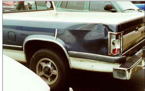
Figure 9: Damage to other vehicle's left back from side slap impact (i.e., 2 nd event) with case vehicle; Note: direct damage begins at white tape
