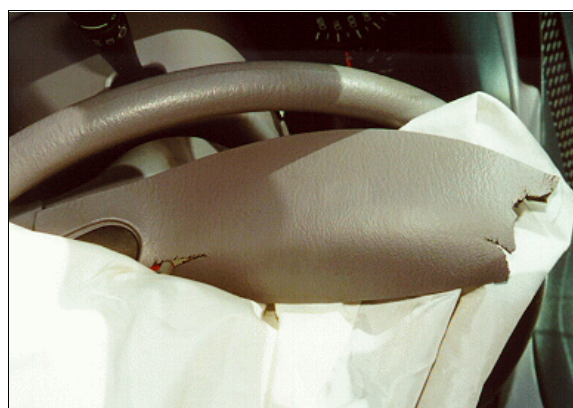
Figure 19: Close-up of right side of case vehicle driver air bag module’s top cover flap showing that part of corner that has been torn away
