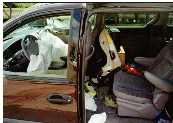
Figure 24: On-scene view of case vehicle's second seating area with unsecured child safety seat leaning forward against front right seat back
