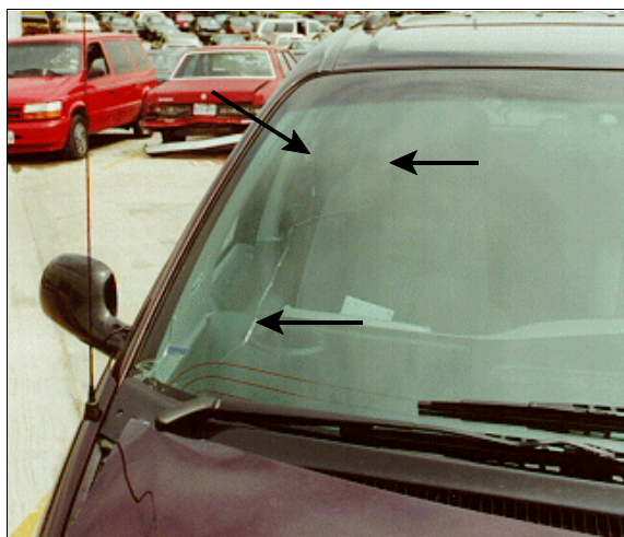
Figure 14: Hairline cracks to case vehicle's right windshield from impact with other vehicle's left front; Note: arrows highlight cracks
