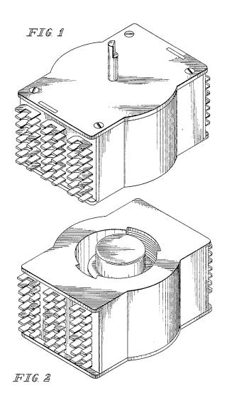
FIGURE 1 is a top perspective view of a housing for a sequential timing device;
