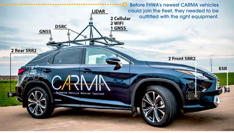
CARMA vehicles are loaded with equipment, including two rear and two front side detection sensors (labelled SRR2), antennas for global navigation satellite systems (GNSS), dedicated short-range communications (DSRC), light detection and ranging (LiDAR), and electronically scanning radar (ESR). Source: FHWA.
