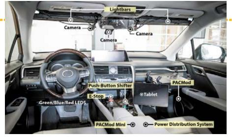
Equipment in the vehicles' interiors includes lightbars and floor LEDs, cameras, a push-button shifter and emergency stop button, a tablet, the power distribution system, and the platform actuation and control module (PACMod and PACMod Mini).
