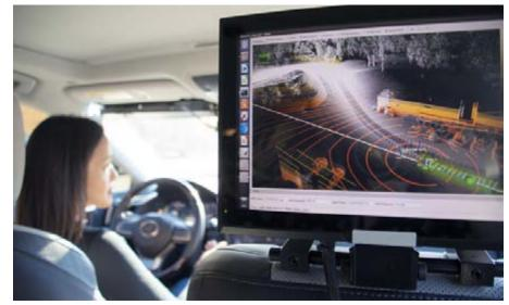
This photo depicts how waypoint following appears on a screen in a CARMA3-equipped vehicle to show localization, which is how CARMA recognizes what is around the vehicle. Source: FHWA
