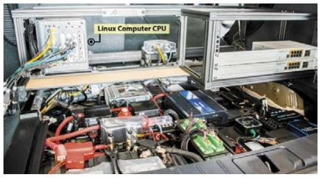
The Linux-based computer housed in the vehicle's trunk runs the speed and steering software. Source: FHWA.
