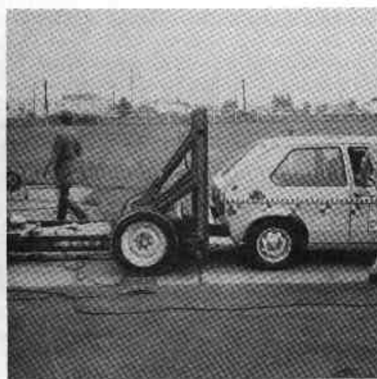
FIGURE 11A VIEW OF MOVING BARRIER
