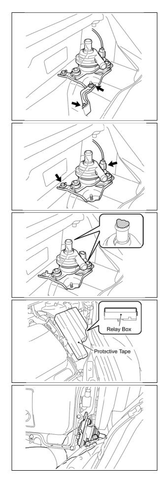
c) Remove the nut, bolt, and bracket.
