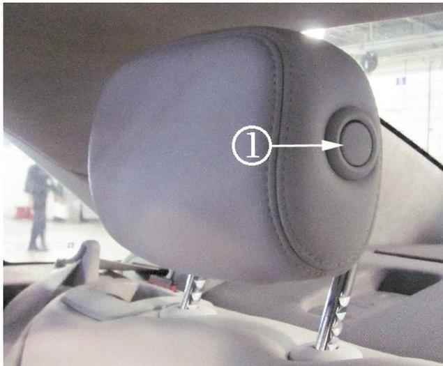
6. Verify that the head restraint release button returns fully from the depressed position.
