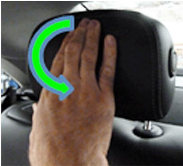
7. Verify that the head restraint is locked into the upright position with a push/pull from the top of the head restraint.
