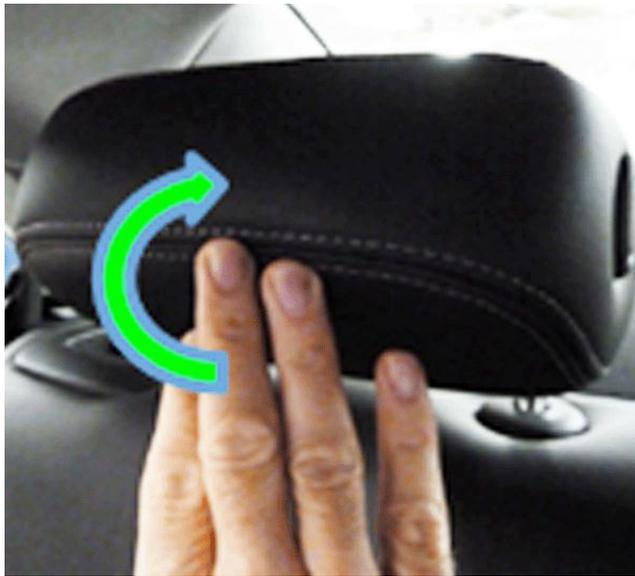
5. Push head restraint into the upright position.
