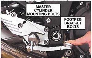
Depress the brake pedal to align the master cylinder bolt holes, install the bolts, and tighten the bolts to 25N·m(2.5 kgf-m, 18ft-lb).
