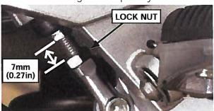
Check for clearance between the rod end and the top of the brake pedal.
