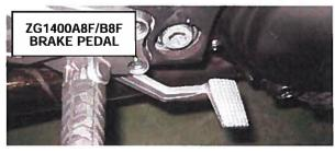
Adjust the rear master cylinder push rod to a length of 7mm (.27in) measured between the two nuts and tighten temporarily.
