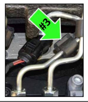
Install fuel line Damper (03L 130 118) in the center of #1 fuel line as shown <arrow>
