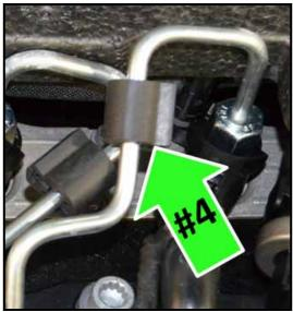
⇐ Install fuel line Damper (03L 130 118) in the center of #3 fuel line as shown <arrow>
