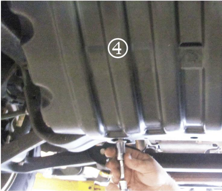
4. Remove the engine shield (4). Refer to *Engine Shield Replacement* in SI.
