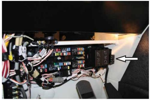
5. Route the jumper harness along the main harness up and around the dash until the mirror switch is reached. Disconnect the mirror switch and connect the new harness between the switch and cab harness.
