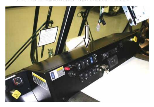
3. Inspect the rear of the mirror switch for signs of overheating. If the switch shows signs of overheating, such as wire insulation melted or discolored, replace the switch with part number 25165161.
