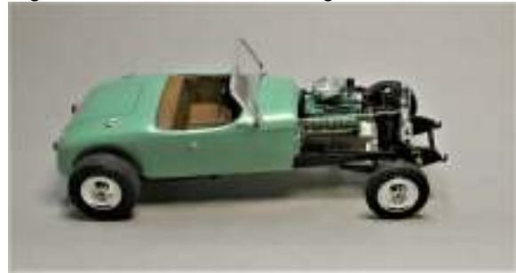
I added the two radiator tie rods made from .020" brass wire
