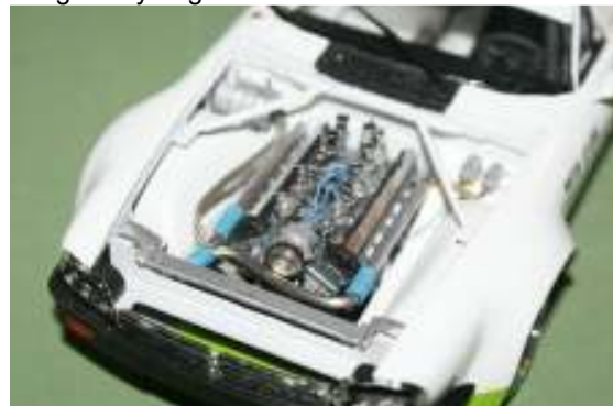
Photo 7: The Weber carbs are from Replicas and Miniatures and the velocity stack are different lengths because the real car had a hood clearance problem. For the blue connections I used heat shrink tubing.
