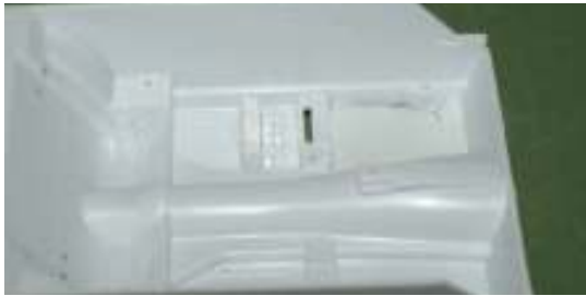
Photo 3: At this point I had cut out the left side details in the existing to make room for the new seat. It was some kind of tank they had in the interior.
