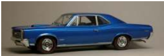
1966 Pontiac Tempest GTO 2 door post body Very rare body style used by drag racers because it was lighter than the hardtop.
