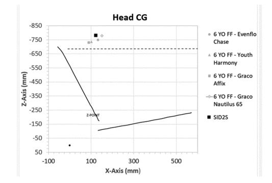
Figure 2. Head CG position of the HIII-6-year-old dummy in booster seats and the SID-IIs 5<sup>th</sup> percentile female dummy in no booster.
