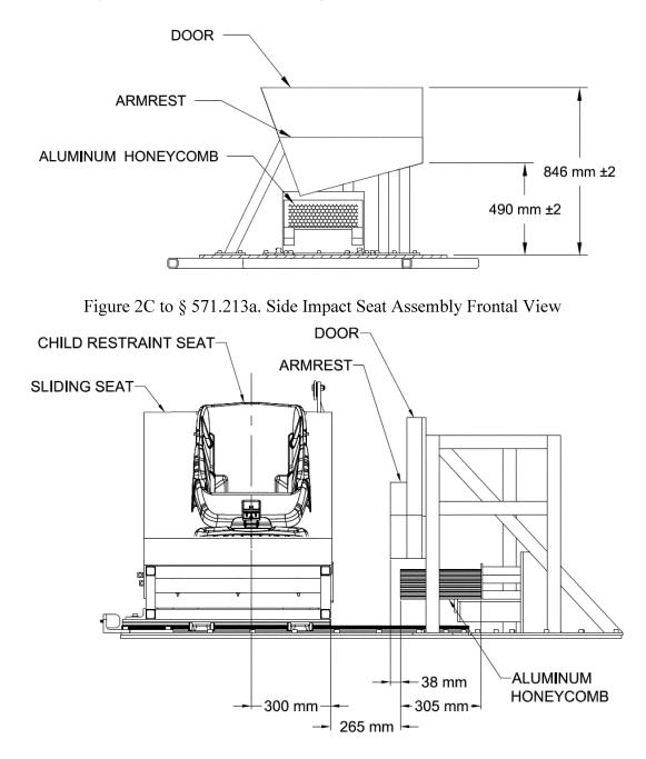
Figure 2D to § 571.213a. Side Impact Seat Assembly Side View
