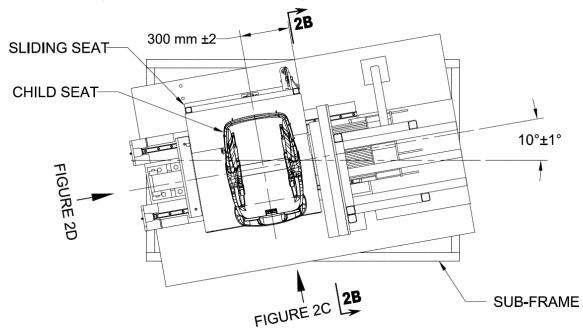
Figure 2B to § 571.213a. Side Impact Seat Assembly Door Panel View
