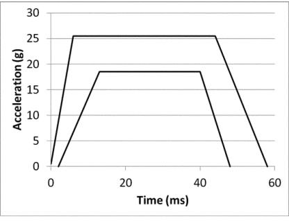
Figure 7 – SISA Bench Seat Acceleration Boundaries (NPRM)
