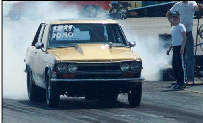
The 1972 Datsun is powered by a 383 Chevrolet stroker small block, a Joe's Transmission powerglide then a Moser rear and runs 10.40's at 130 mph on a good day. "Scott (Conrad) did a lot of work in the off season to improve air flow through the combustion chamber and picked us up about a 1/10th and 1.5 mph... and that really helped racing the stripe!"
