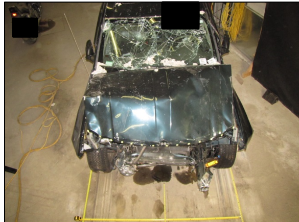
Figure 11: Overhead view of the Jeep's frontal damage.
