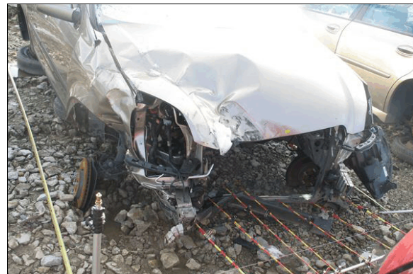
Figure 3: Damage to the front plane of the Honda from the impact with the right plane of the Geo
