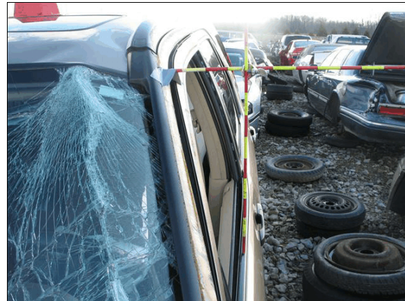
Figure 6: The maximum lateral crush to the Honda's roof structure occurred at the top of the left A-pillar
