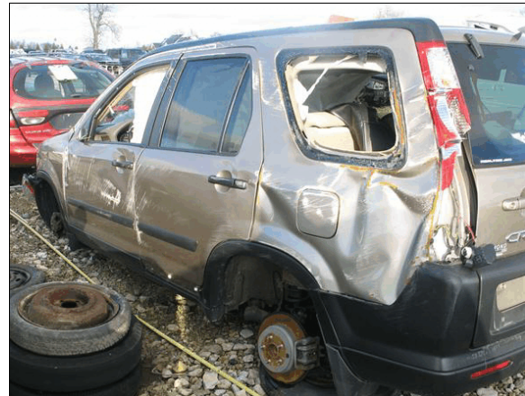
Figure 5: Damage to the left plane of the Honda from the rollover
