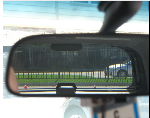
Figure 7: Image through the center mirror to the reference targets positioned aft of the Hyundai.
