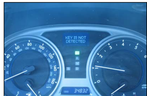
Figure 4: Warning message displayed by the Lexus when the key fob is removed from the running vehicle.
