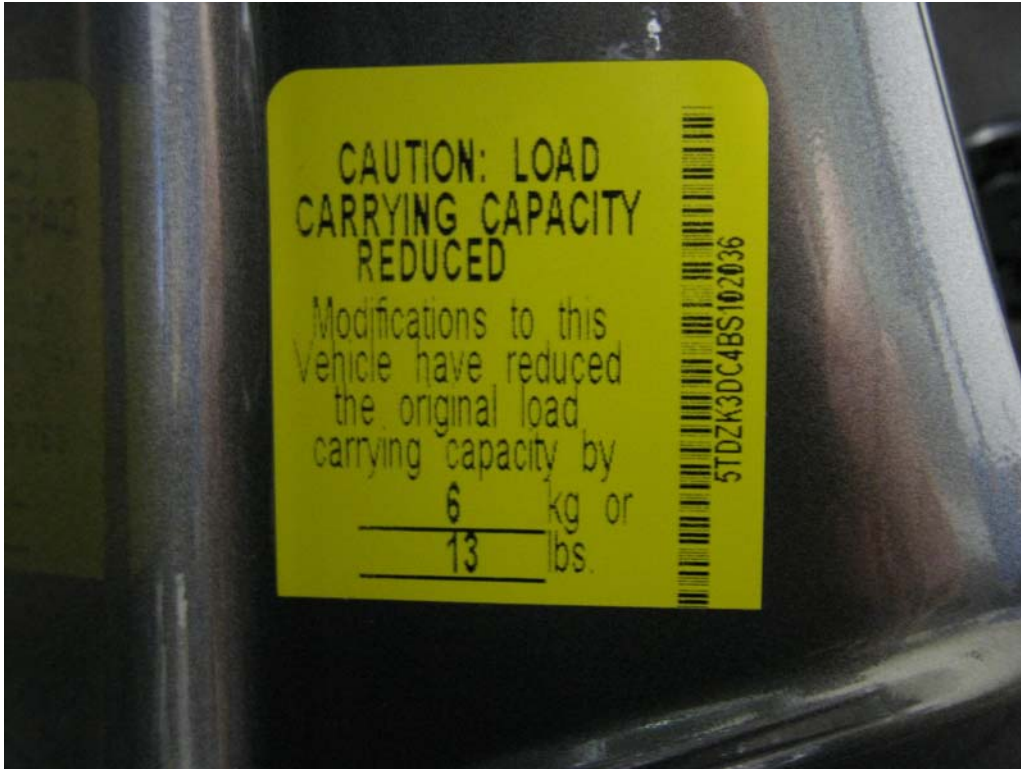
As Delivered – Vehicle’s Caution Load Carrying Capacity Label
