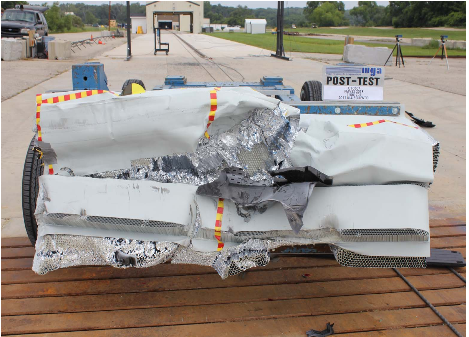
Post-Test Front View of MDB
