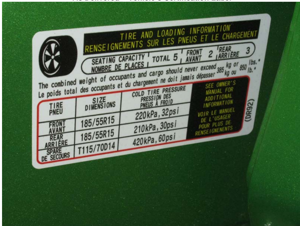
As Delivered – Vehicle’s Tire Information Label
