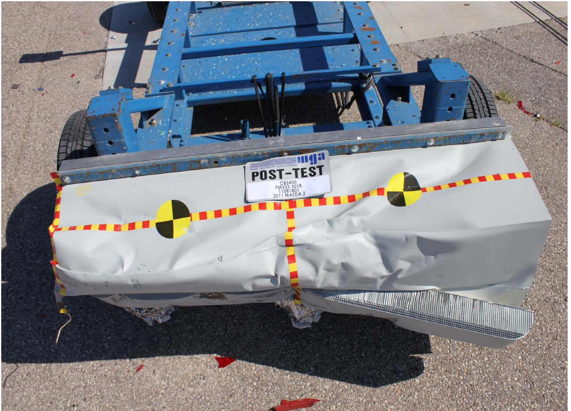
Post-Test Top View of MDB
