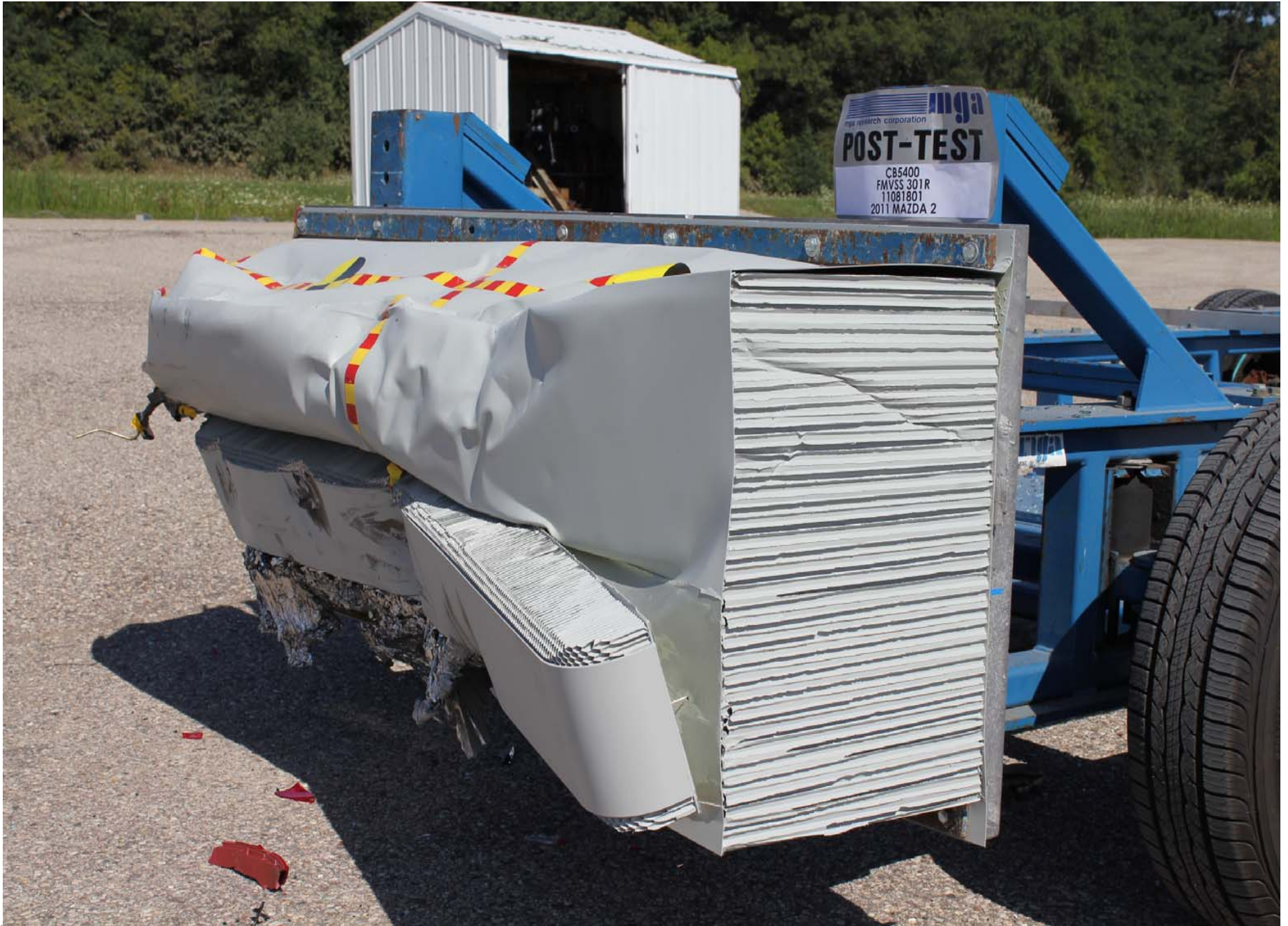
Post-Test \frac{3}{4} Left Side View of MDB
