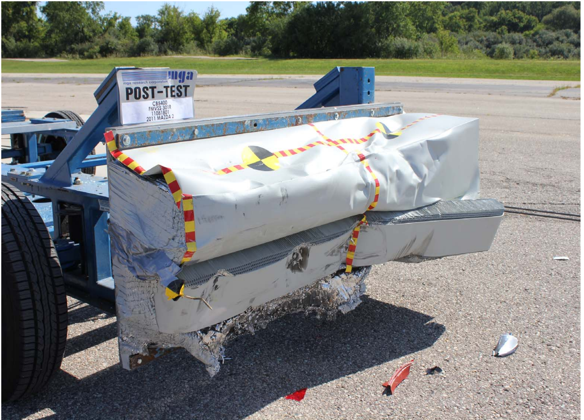
Post-Test ¾ Right Side View of MDB
