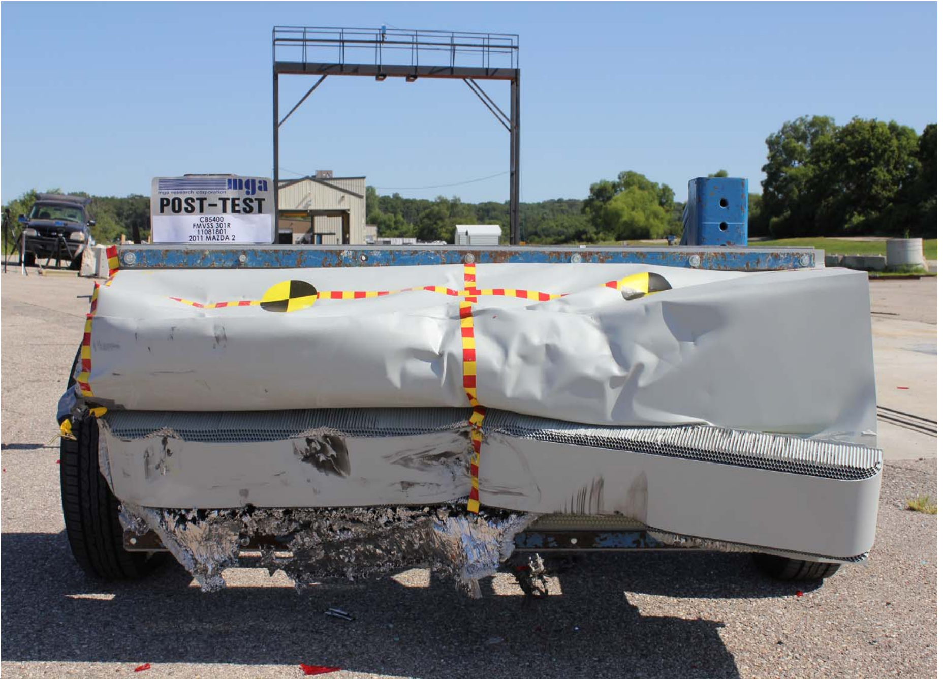
Post-Test Front View of MDB
