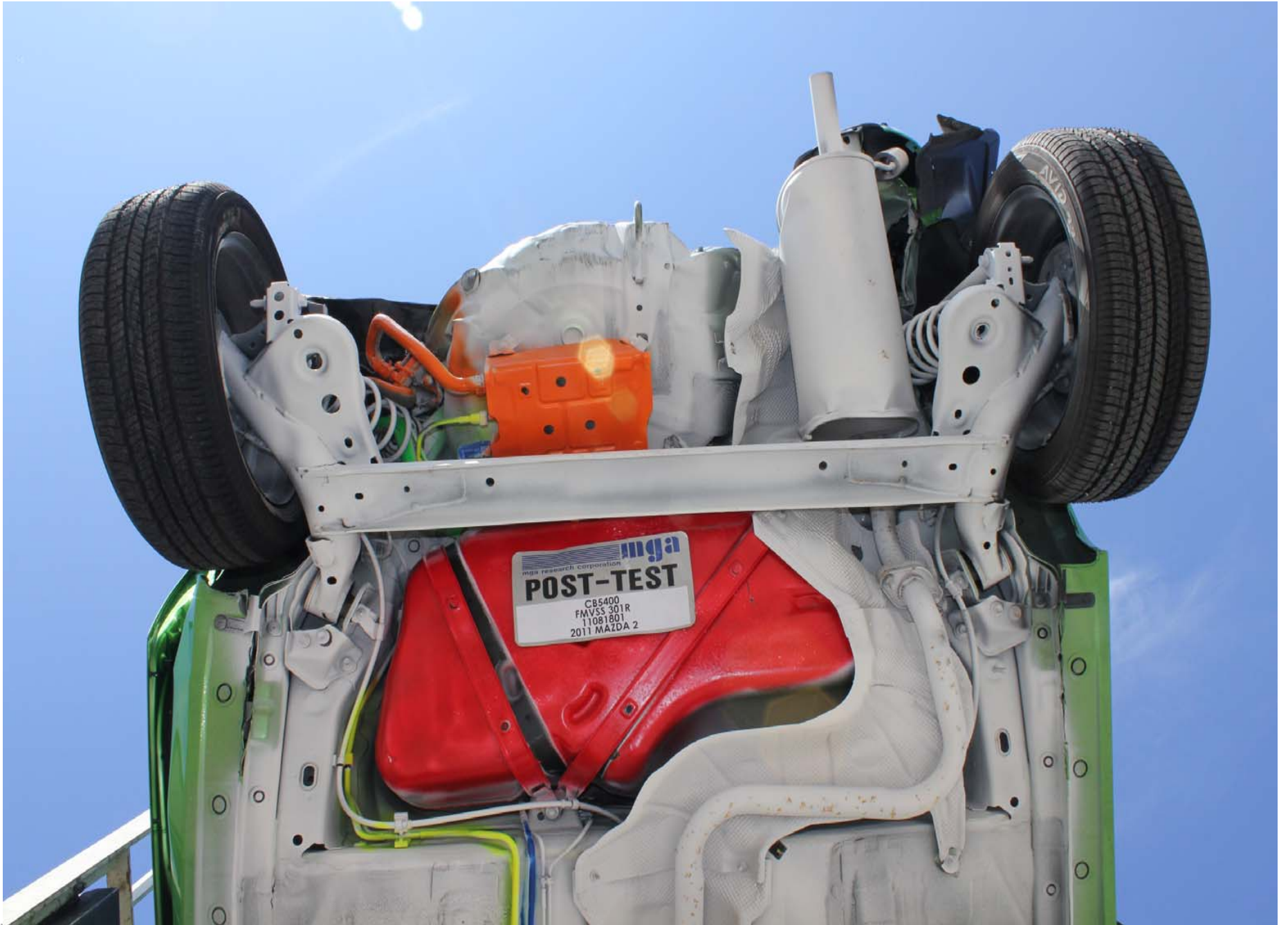
Post-Test Underbody View 3
