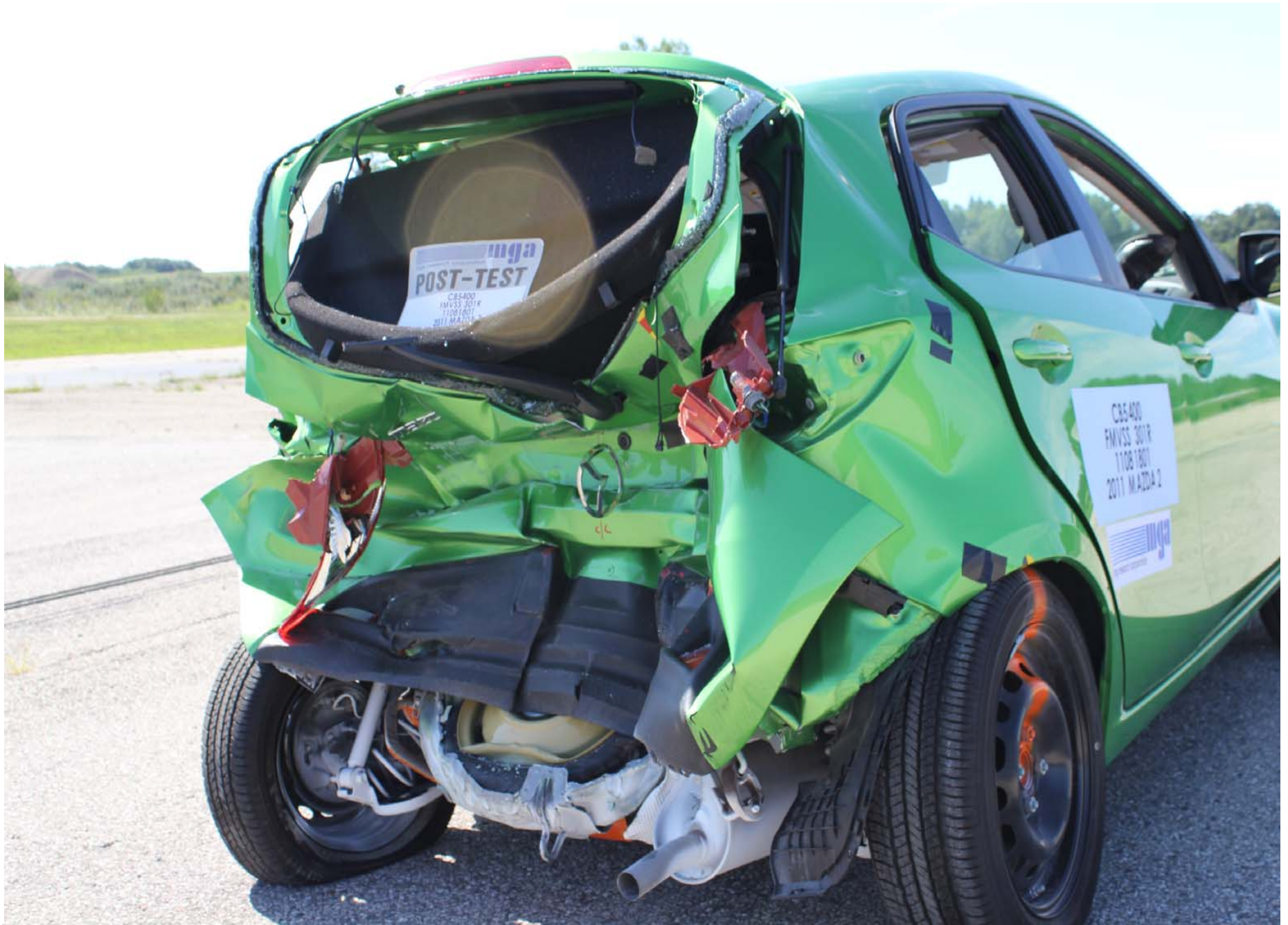
Post-Test Right Rear Close-up View of Vehicle
