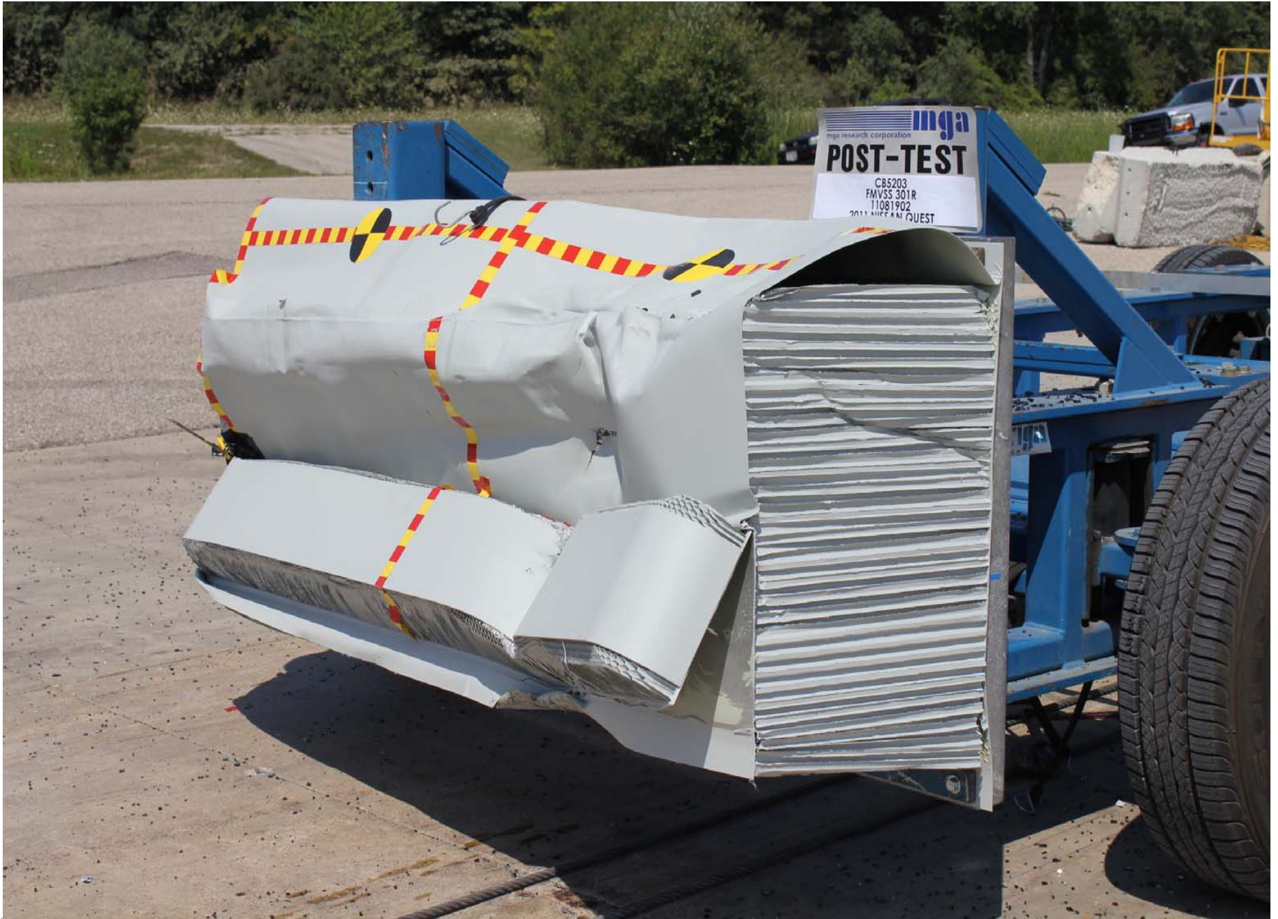
Post-Test \frac{3}{4} Left Side View of MDB
