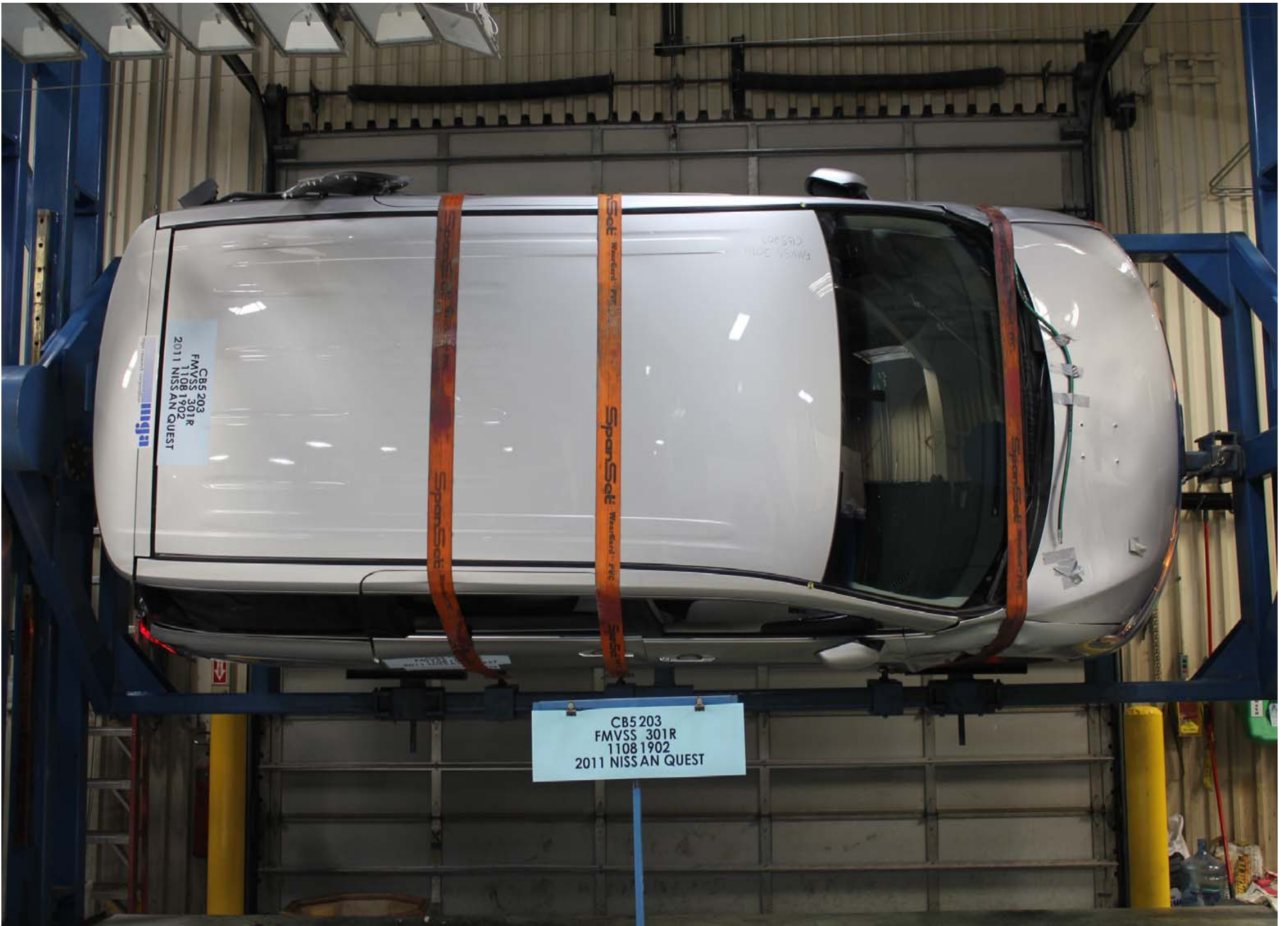
Static Rollover at 270 Degrees
