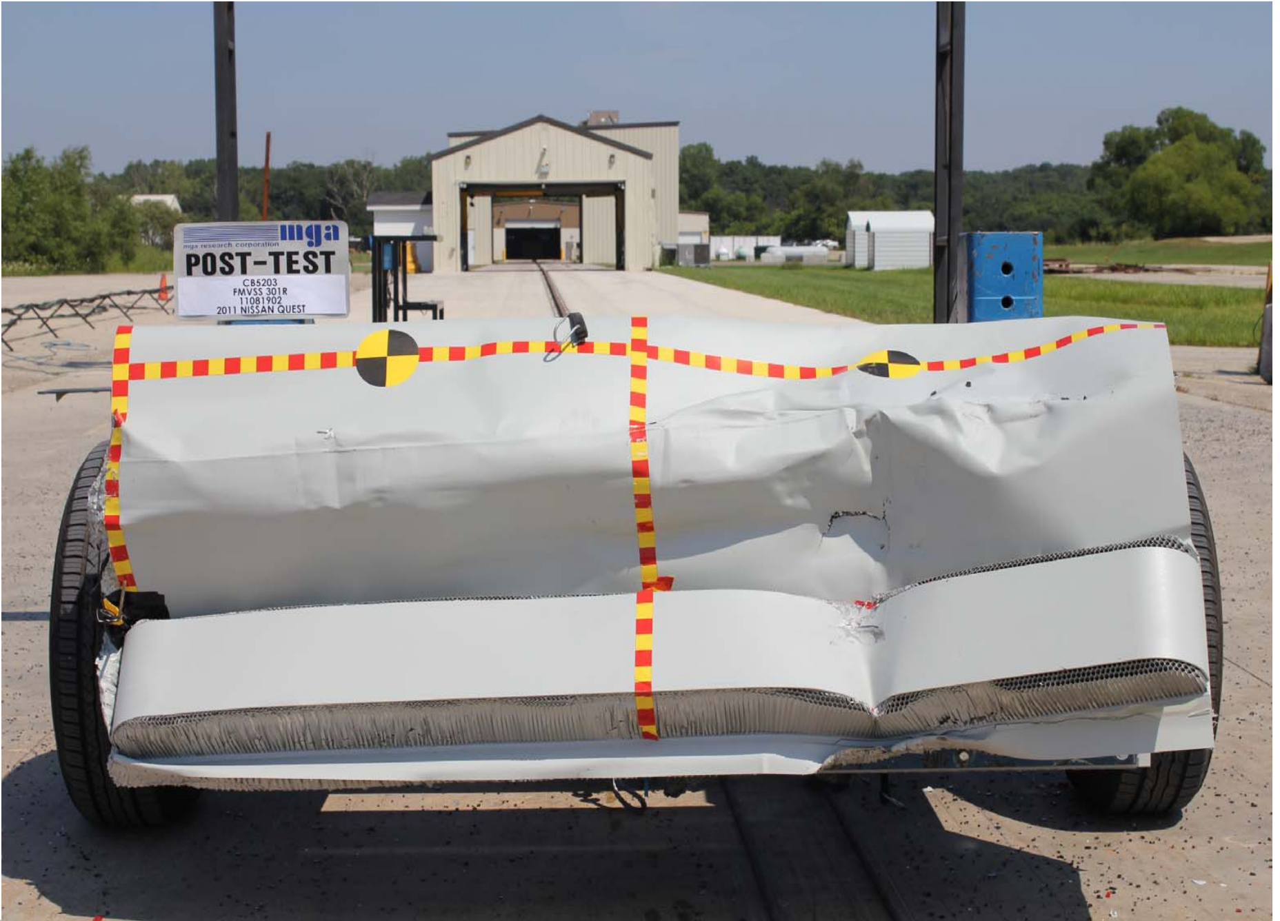
Post-Test Front View of MDB
