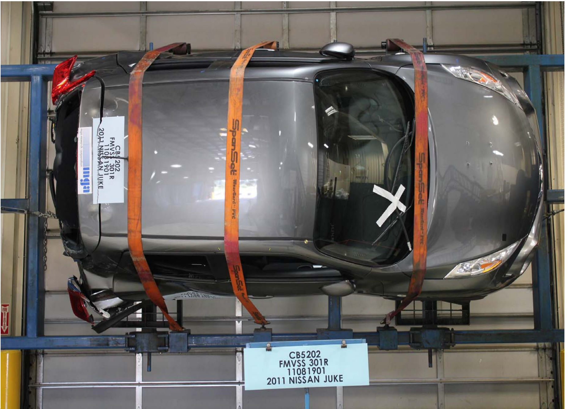
Static Rollover at 90 Degrees
