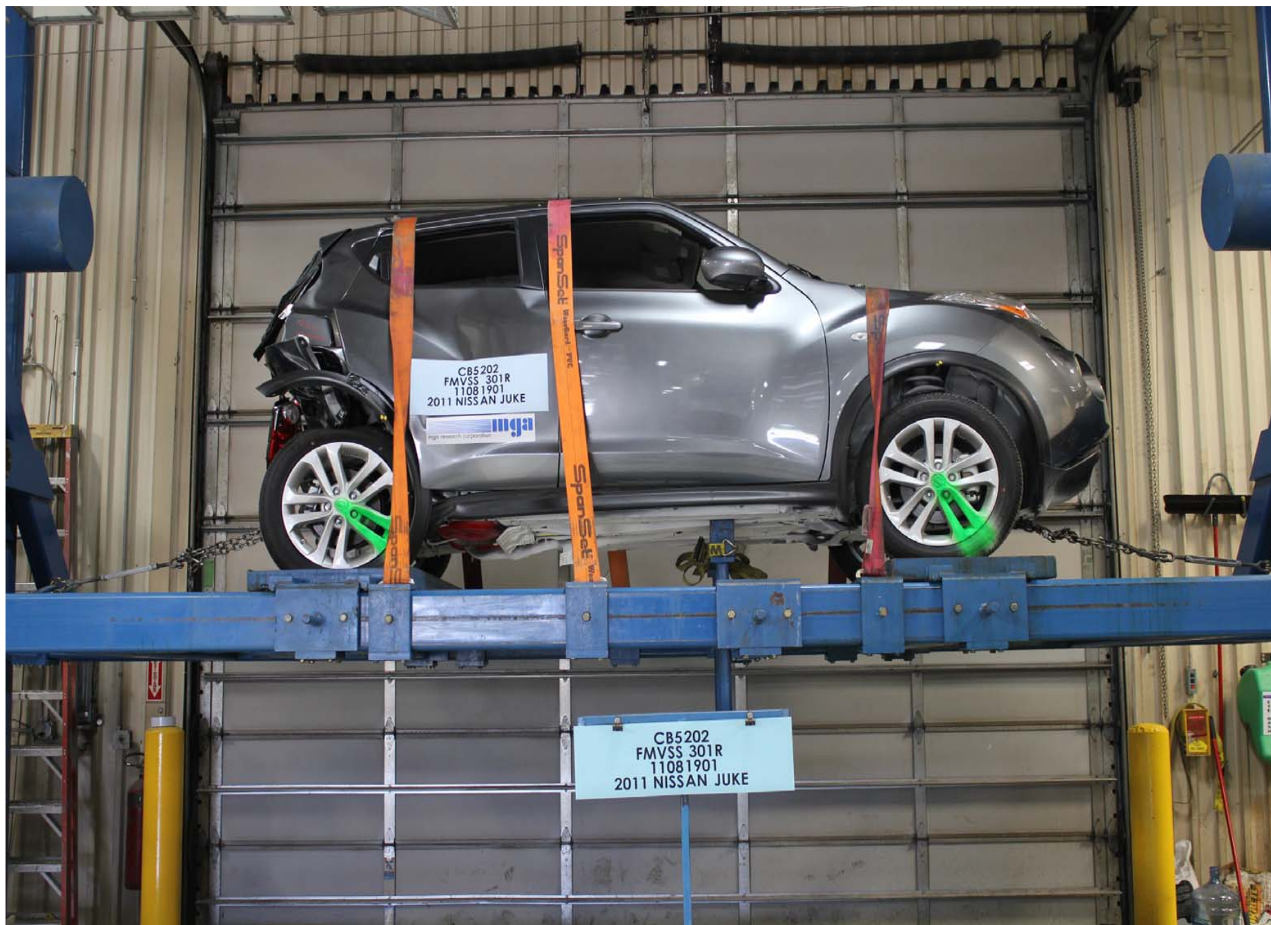
Static Rollover at 360 Degrees
