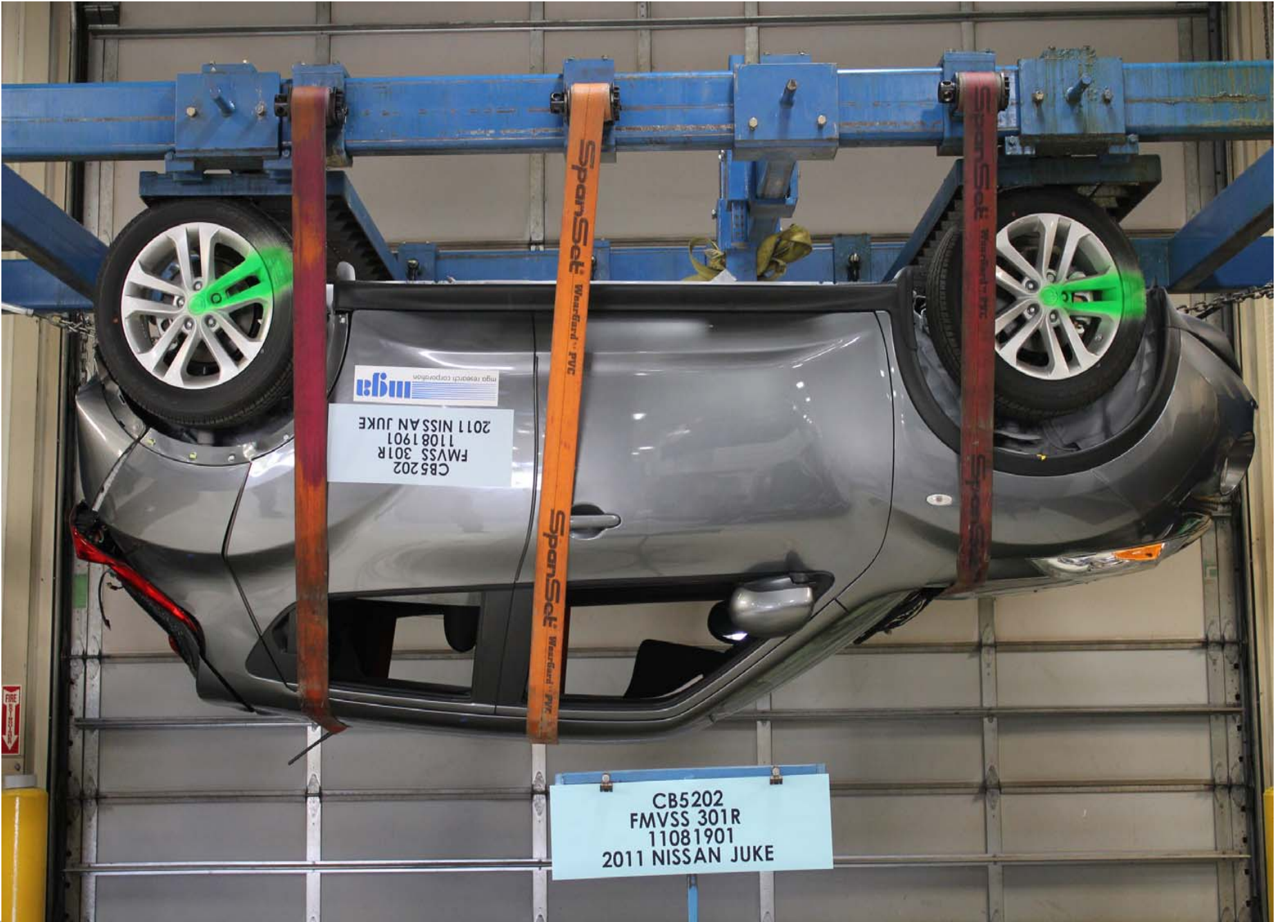
Static Rollover at 180 Degrees
