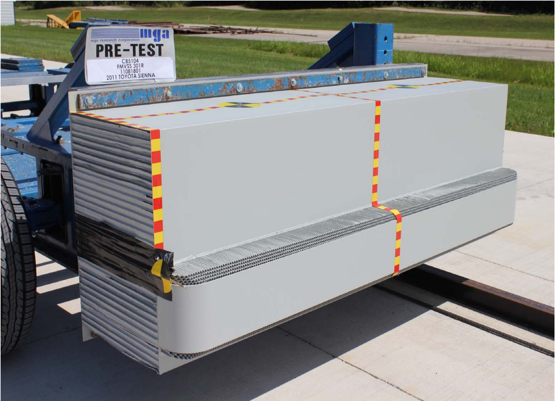
Pre-Test \frac{3}{4} Right Side View of MDB
