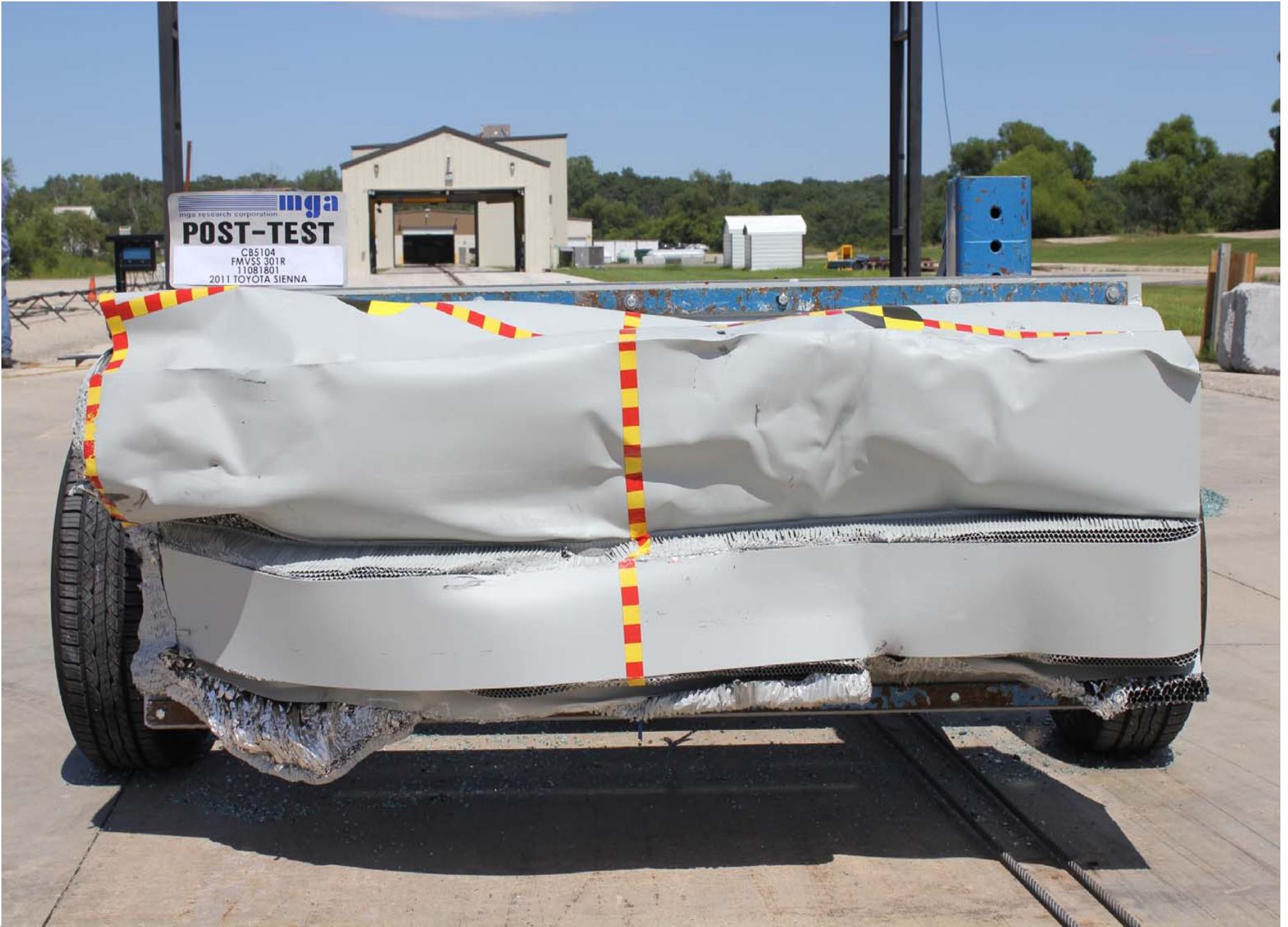
Post-Test Front View of MDB
