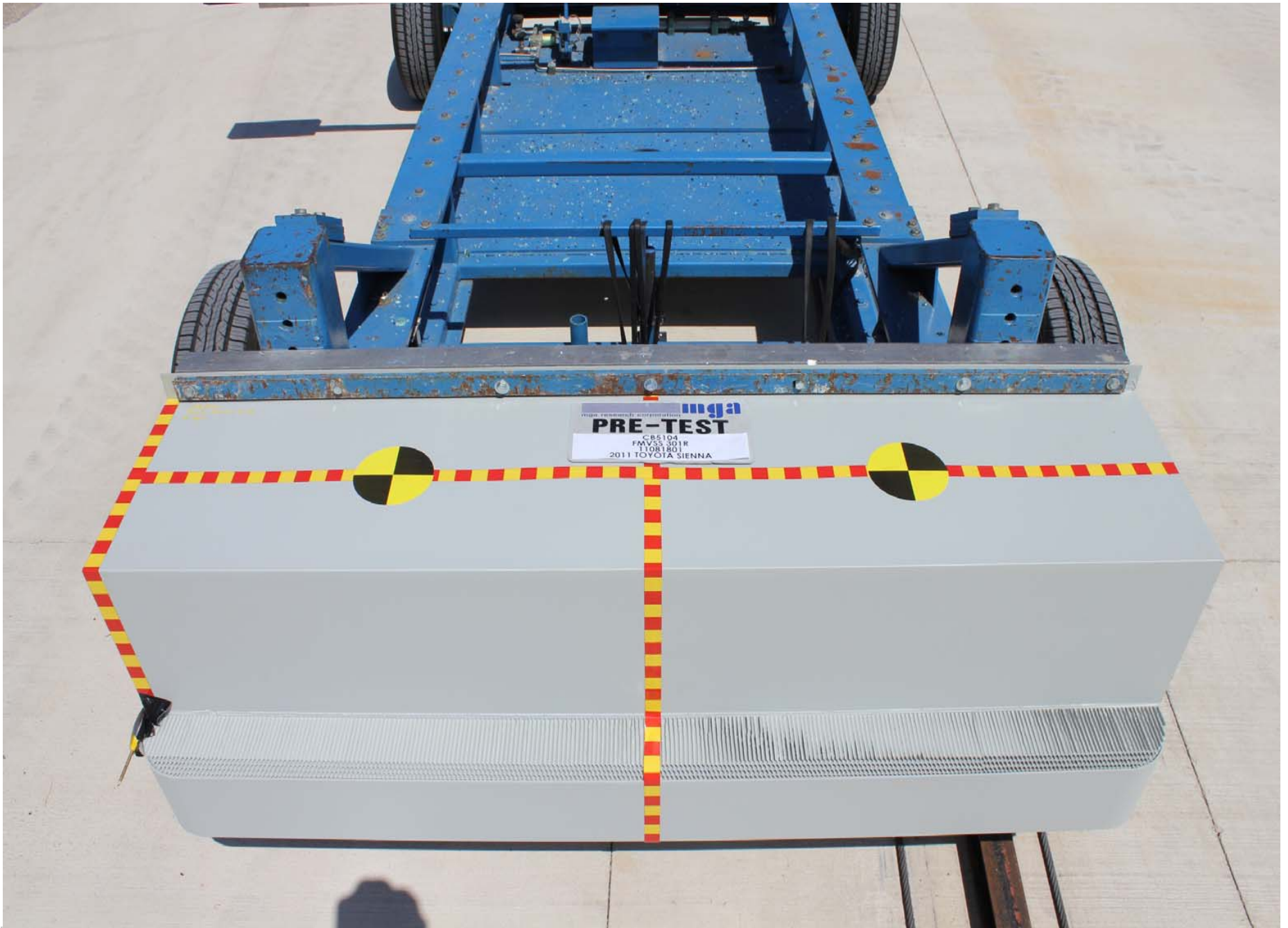
Pre-Test Top View of MDB
