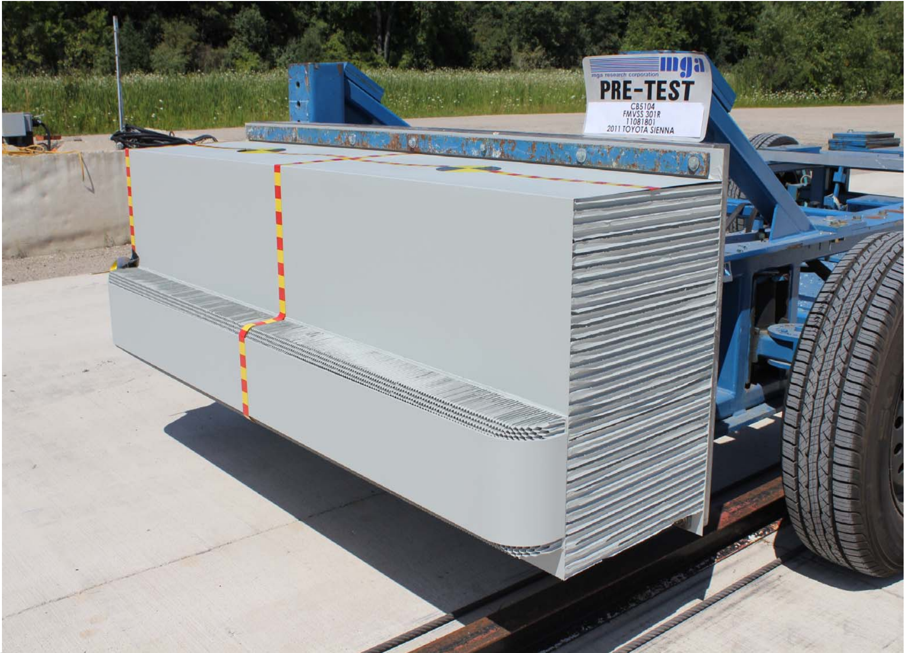
Pre-Test ¾ Left Side View of MDB
