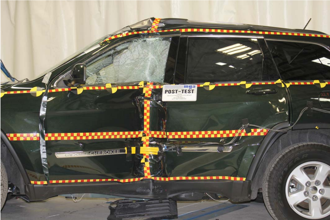
Post-Test Impact Zone Close-up View
