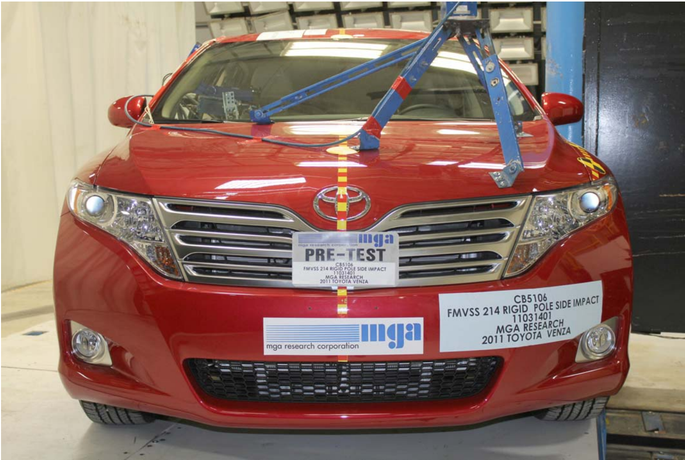
Pre-Test Frontal View of Test Vehicle
