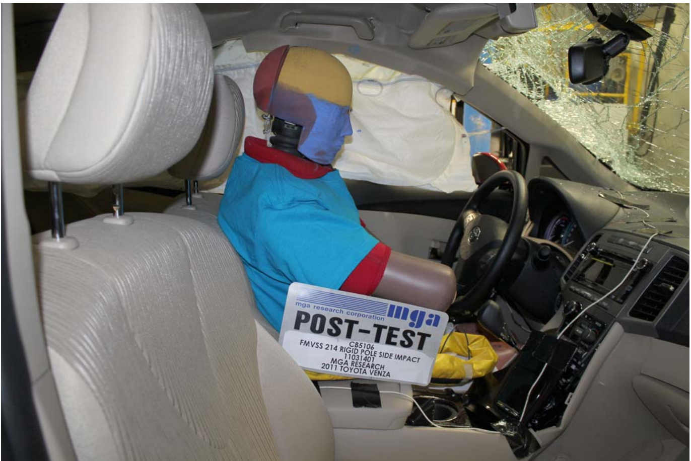
Post-Test Dummy Through Opposite Window
