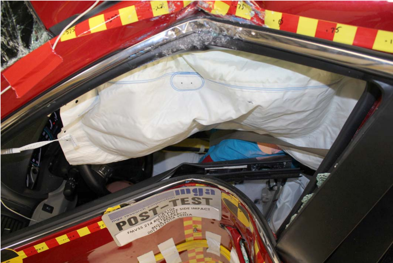
Post-Test Dummy Shoulder and Door Top View
