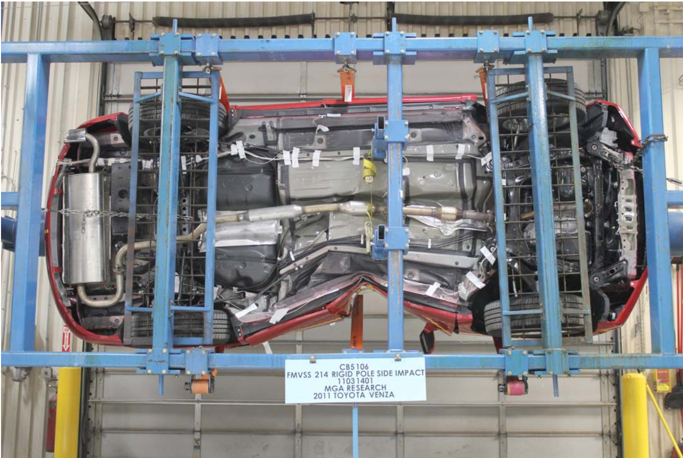
Post-Test Vehicle at 90 Degree Rollover
