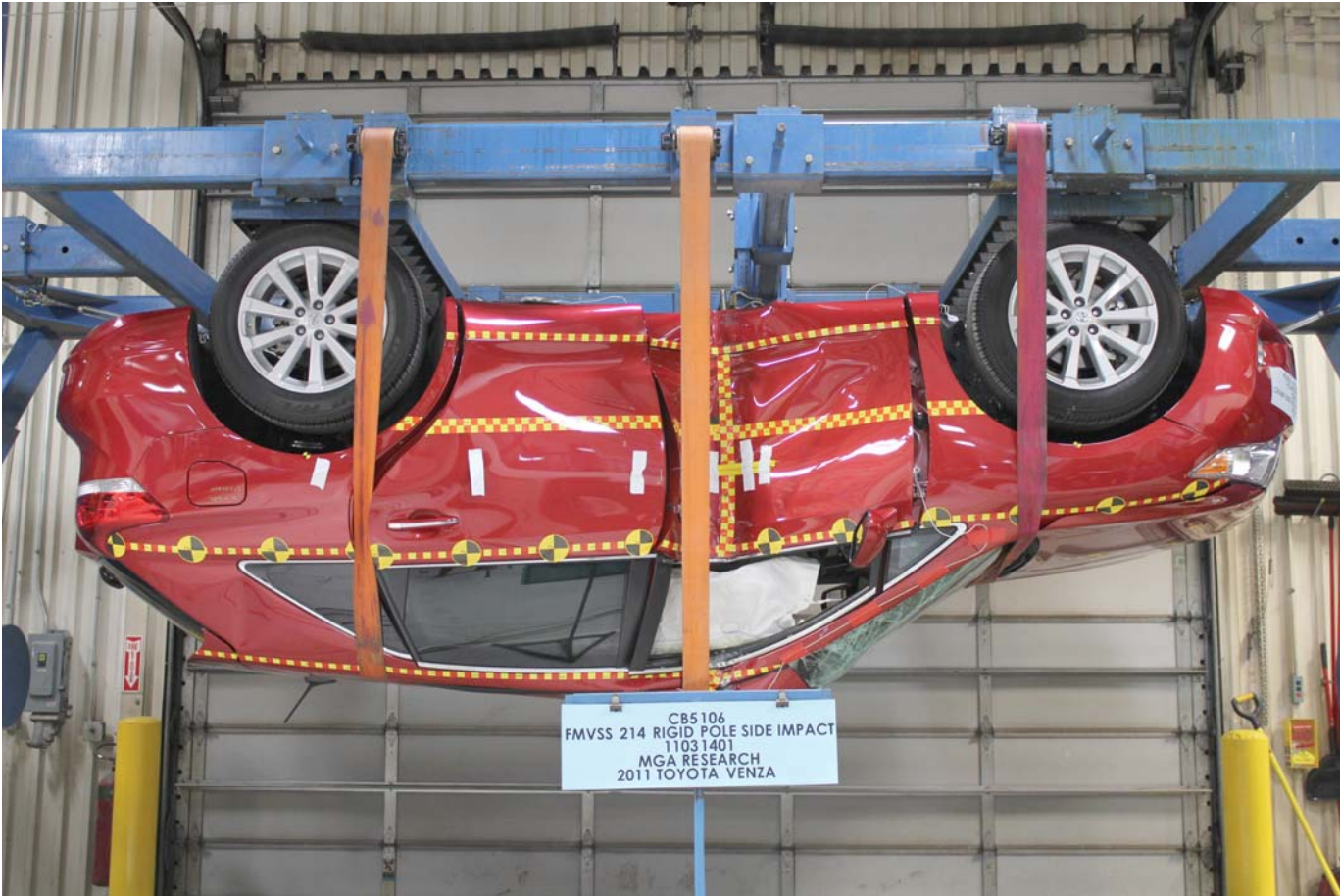
Post-Test Vehicle at 180 Degree Rollover
