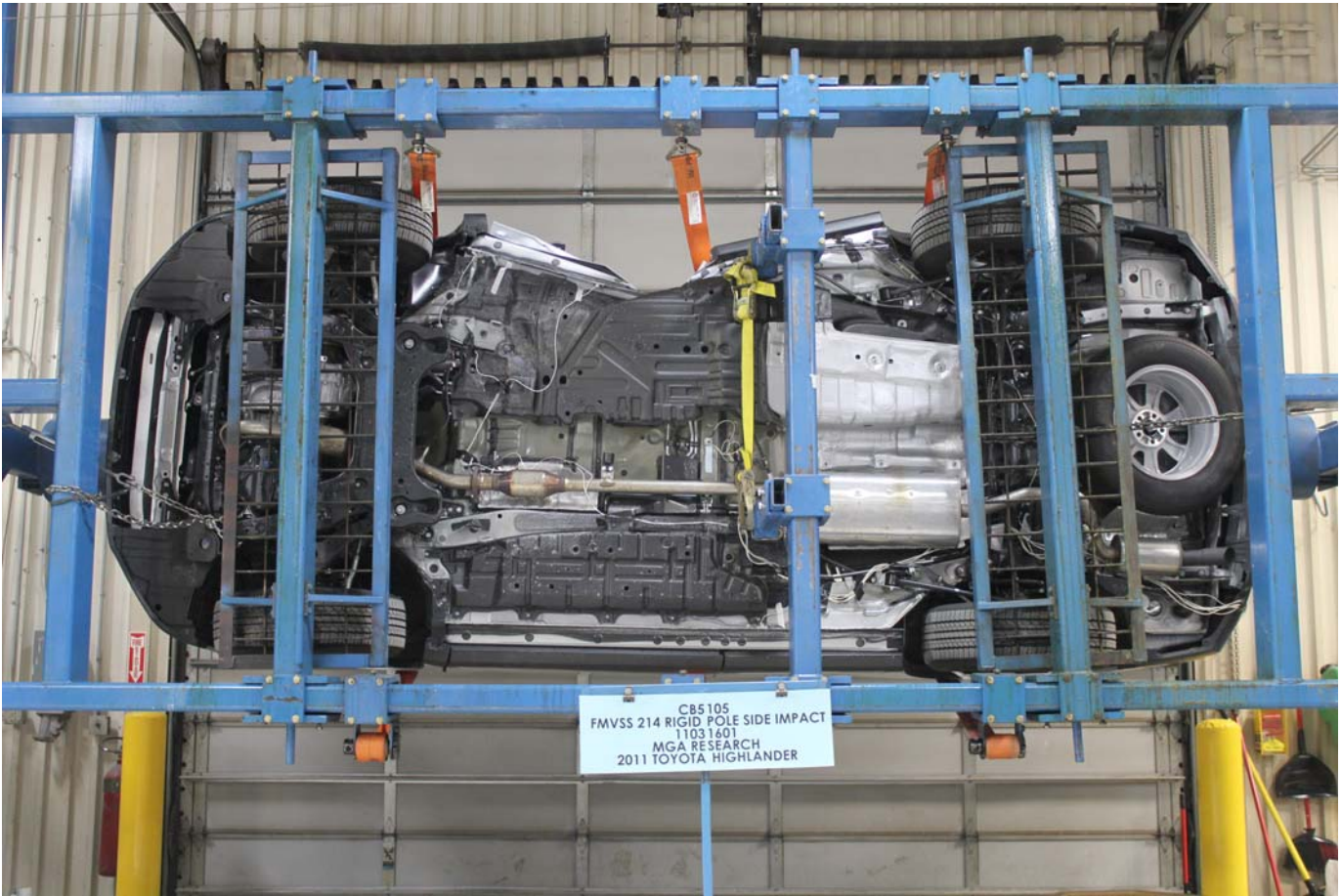
Post-Test Vehicle at 270 Degree Rollover
