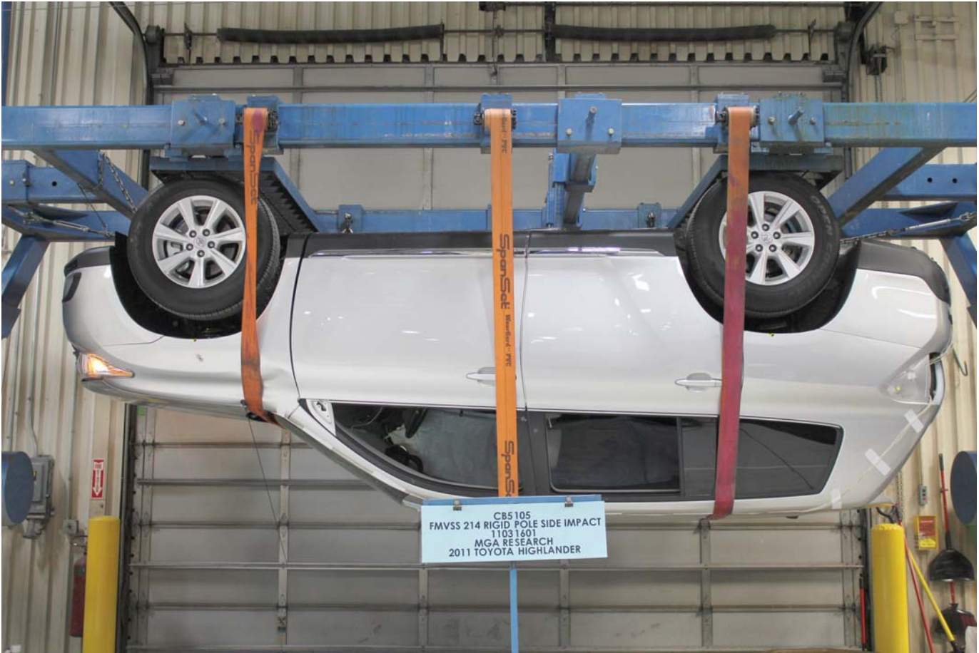
Post-Test Vehicle at 180 Degree Rollover
