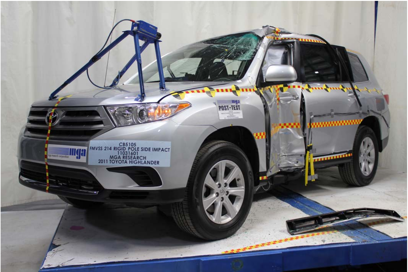
Post-Test \frac{3}{4} Front View of Impact Zone
