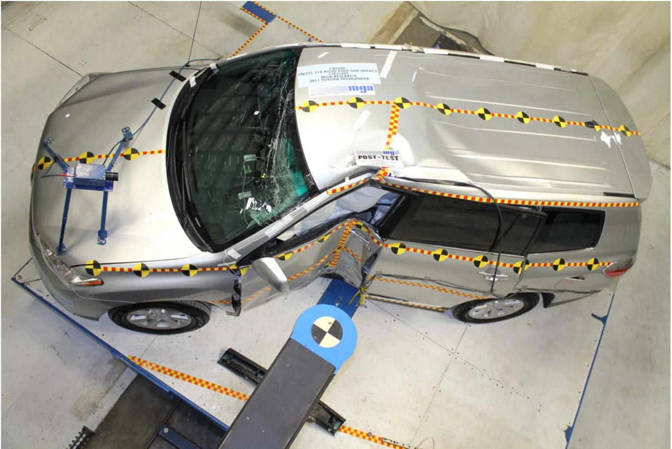
Post-Test Overhead View of Test Vehicle
