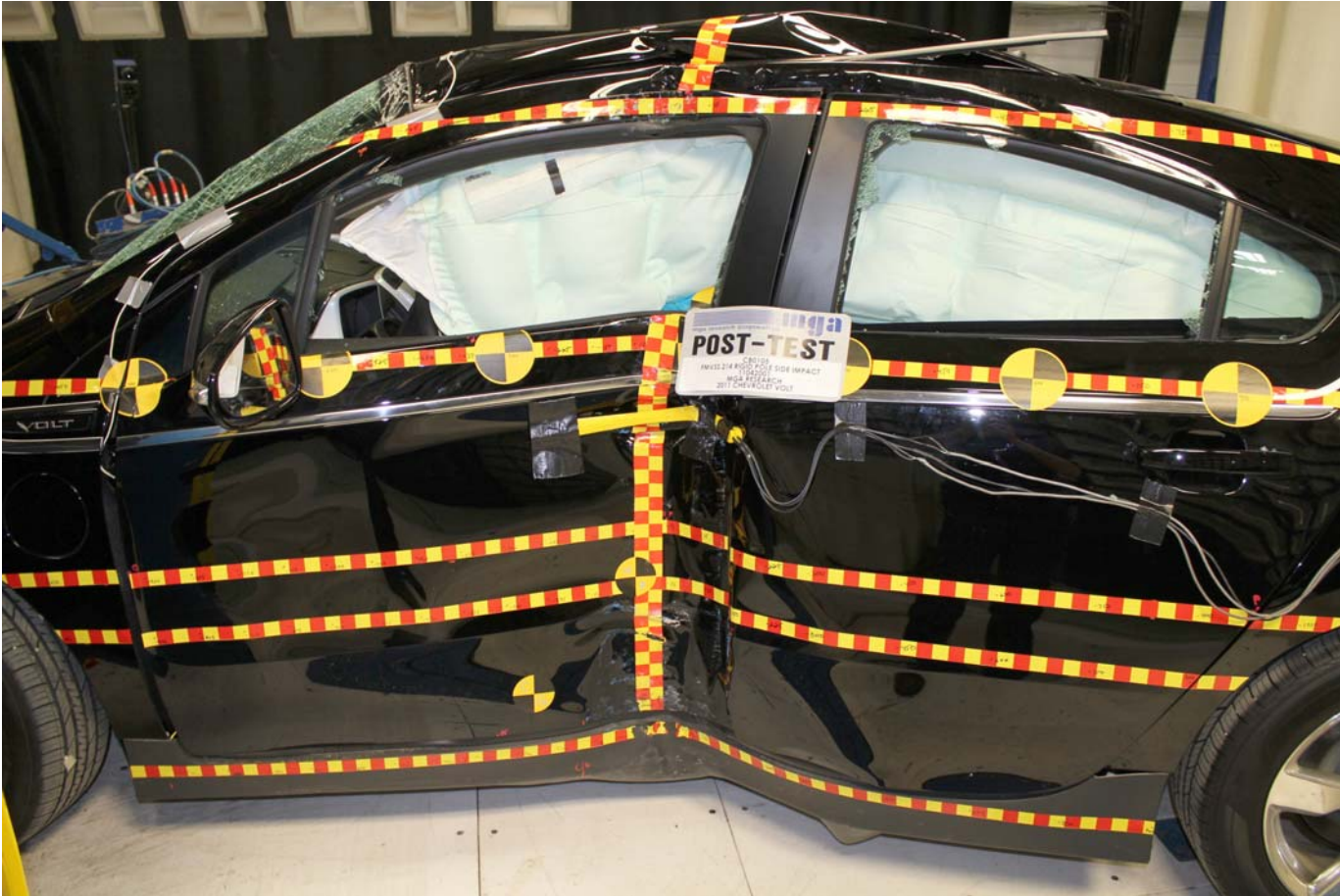
Post-Test Impact Zone Close-up View
