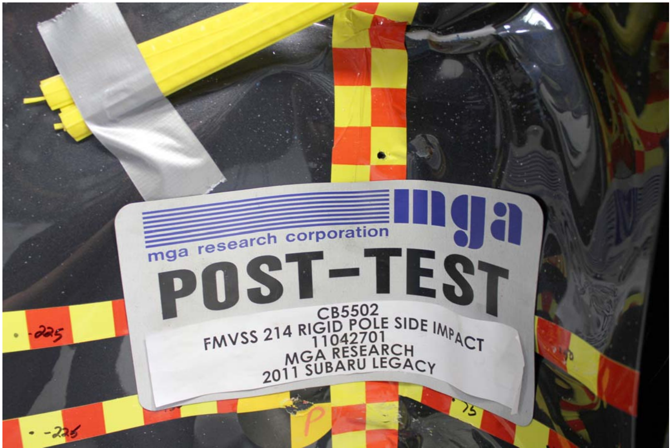
Post-Test Close-up View of Impact Point Target
