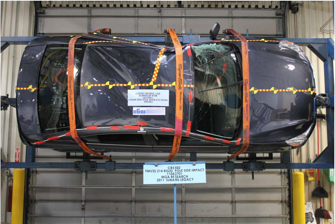
Post-Test Vehicle at 90 Degree Rollover
