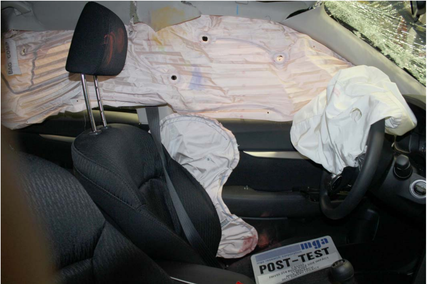
Post-Test Interior of Front Door Showing Dummy Impact Locations
