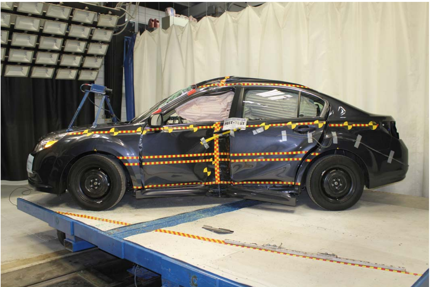
Post-Test Impacted Side View of Test Vehicle
