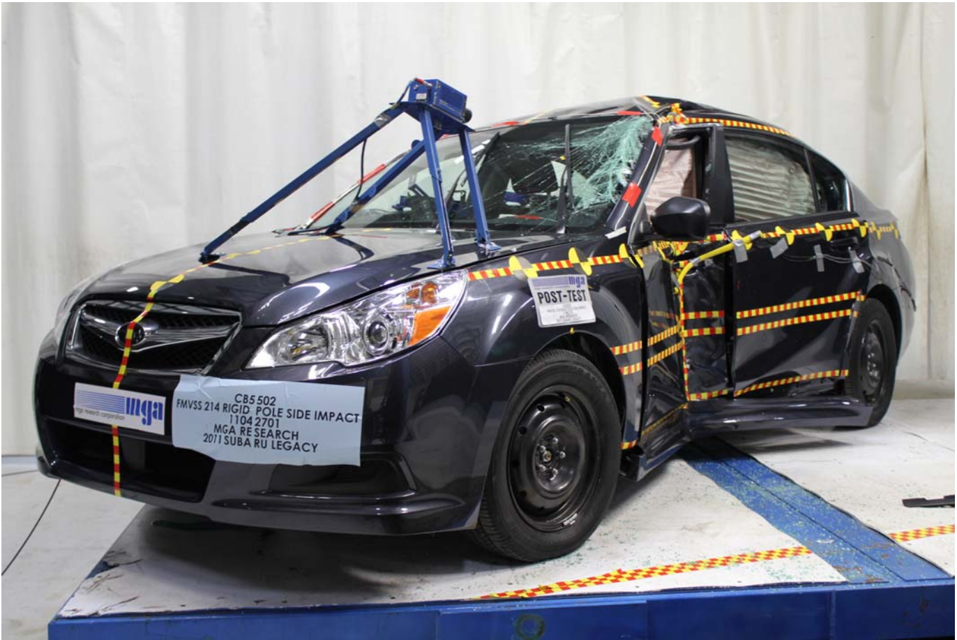
Post-Test \frac{3}{4} Front View of Impact Zone
