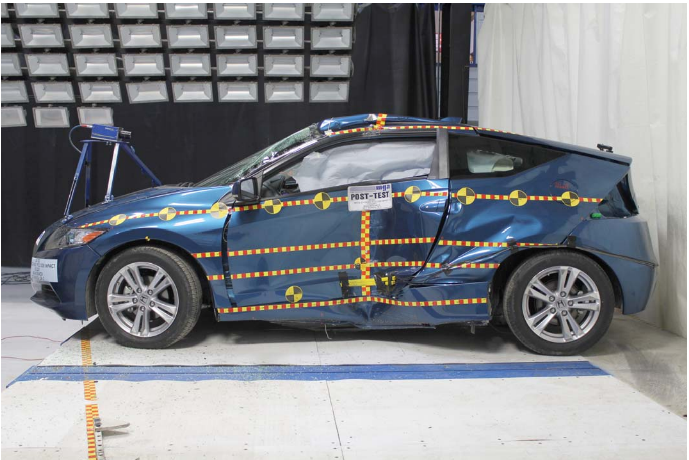
Post-Test Impacted Side View of Test Vehicle
