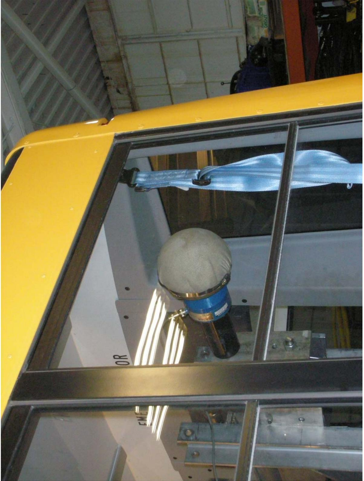
Retention Test of Left Rearmost Upper Window (Pre-Test)
