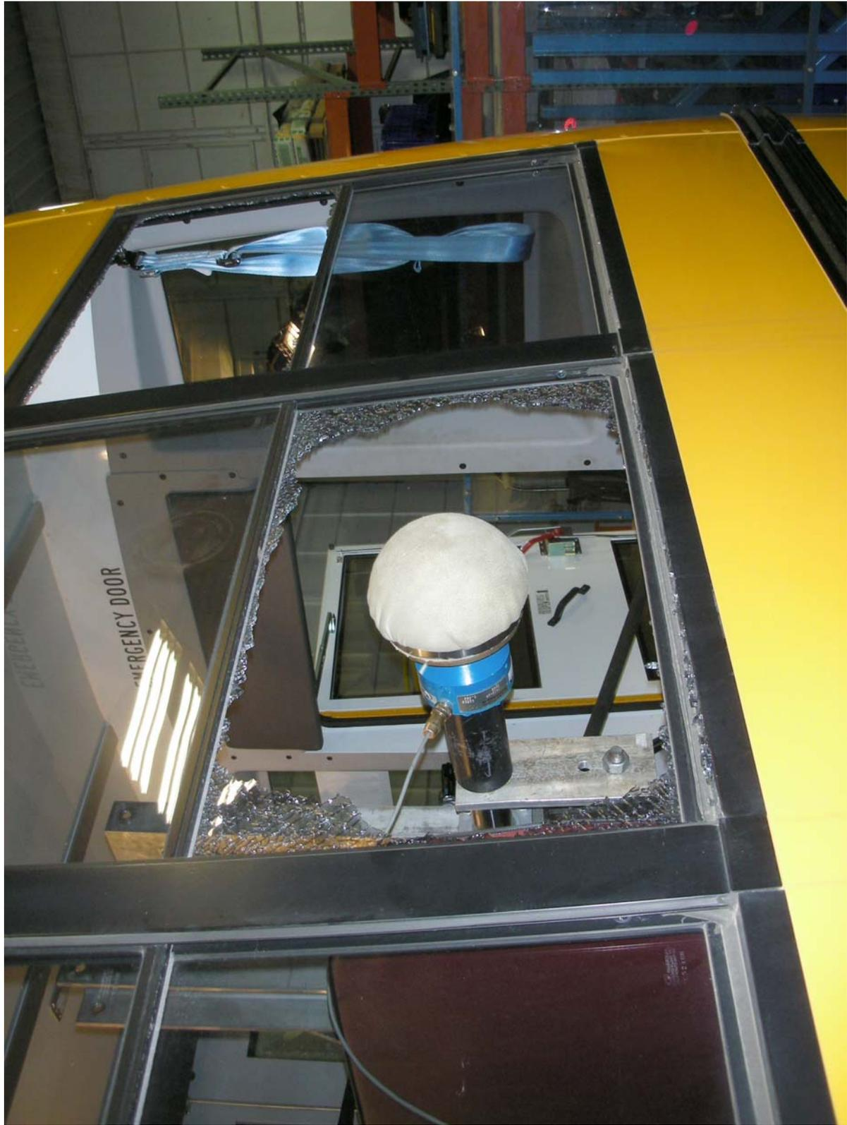
Retention Test of Left Side 4<sup>th</sup> of 5 Lower Window (Post-Test)
