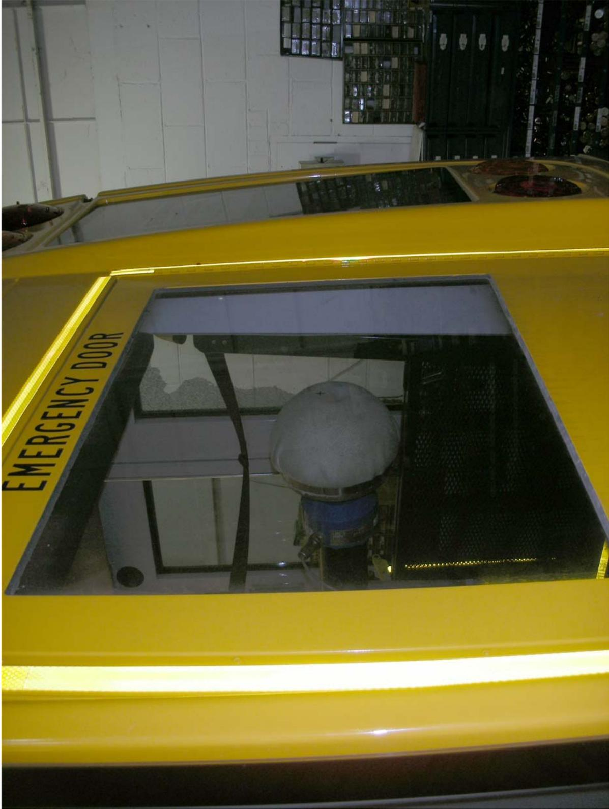
Retention Test of Rear Emergency Door Upper Window (Pre-Test)
