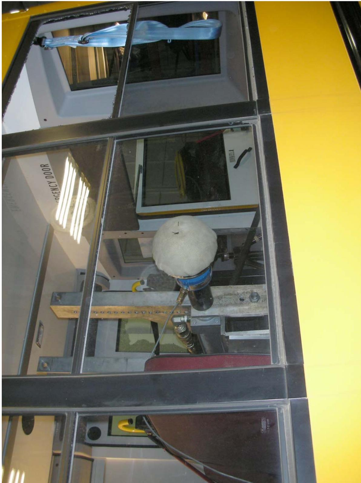
Retention Test of Left Side 4<sup>th</sup> of 5 Lower Window (Pre-Test)
