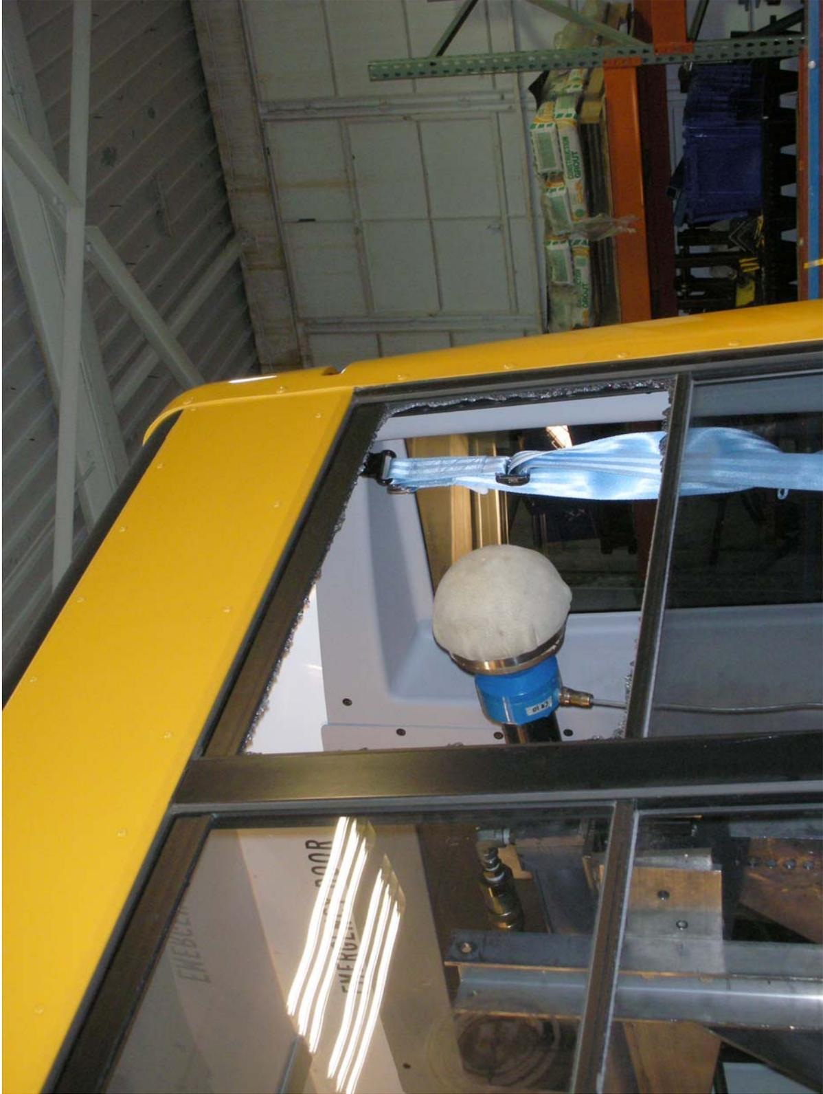
Retention Test of Left Rearmost Upper Window (Post-Test)
