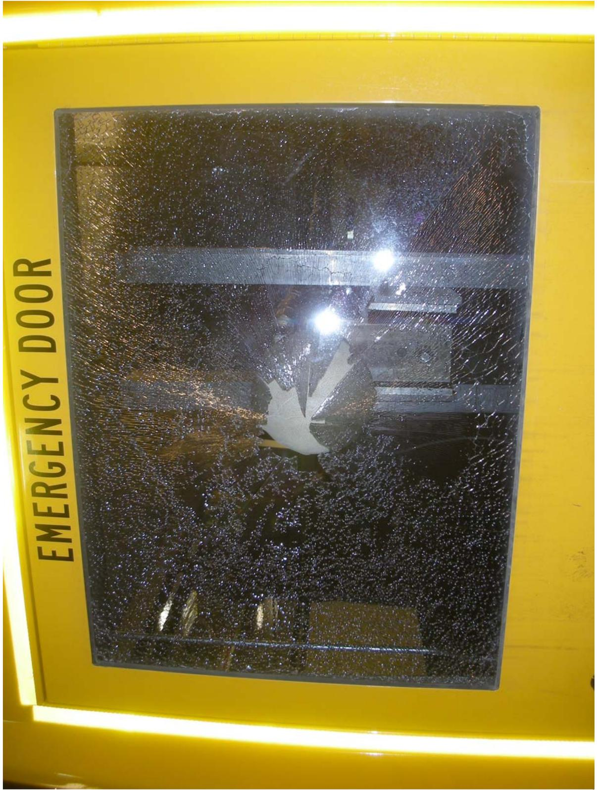
Retention Test of Rear Emergency Door Upper Window (Post-Test)
