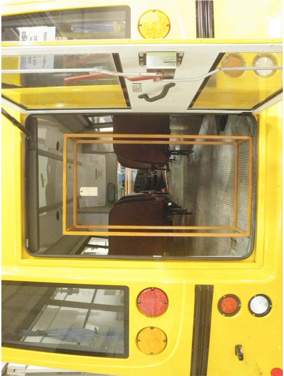
Rear Door Emergency Exit Parallelepiped Clearance
