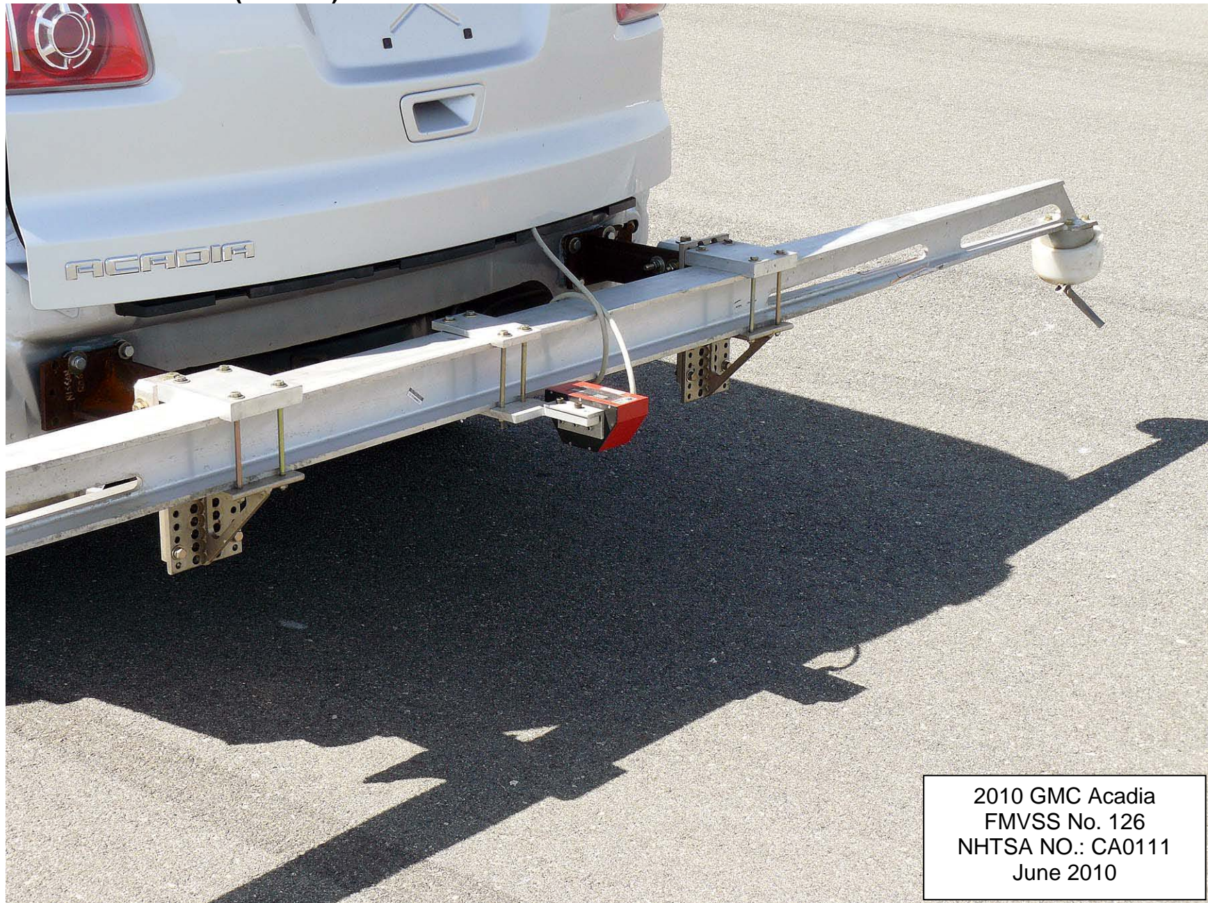
Figure 5.11. Rear Outrigger, Mount and Speed Sensor
