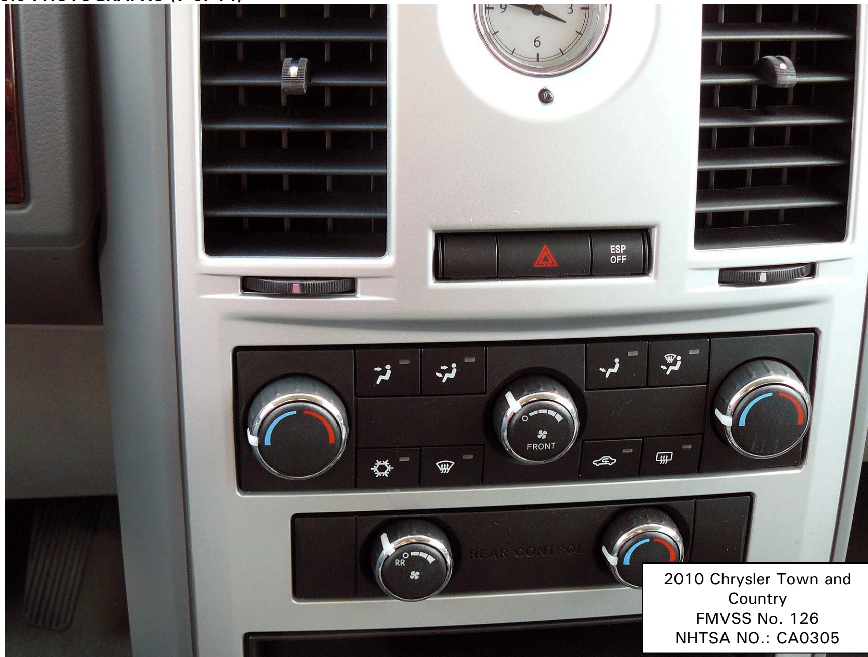
Figure 5.7. ESC Off Control Switch
