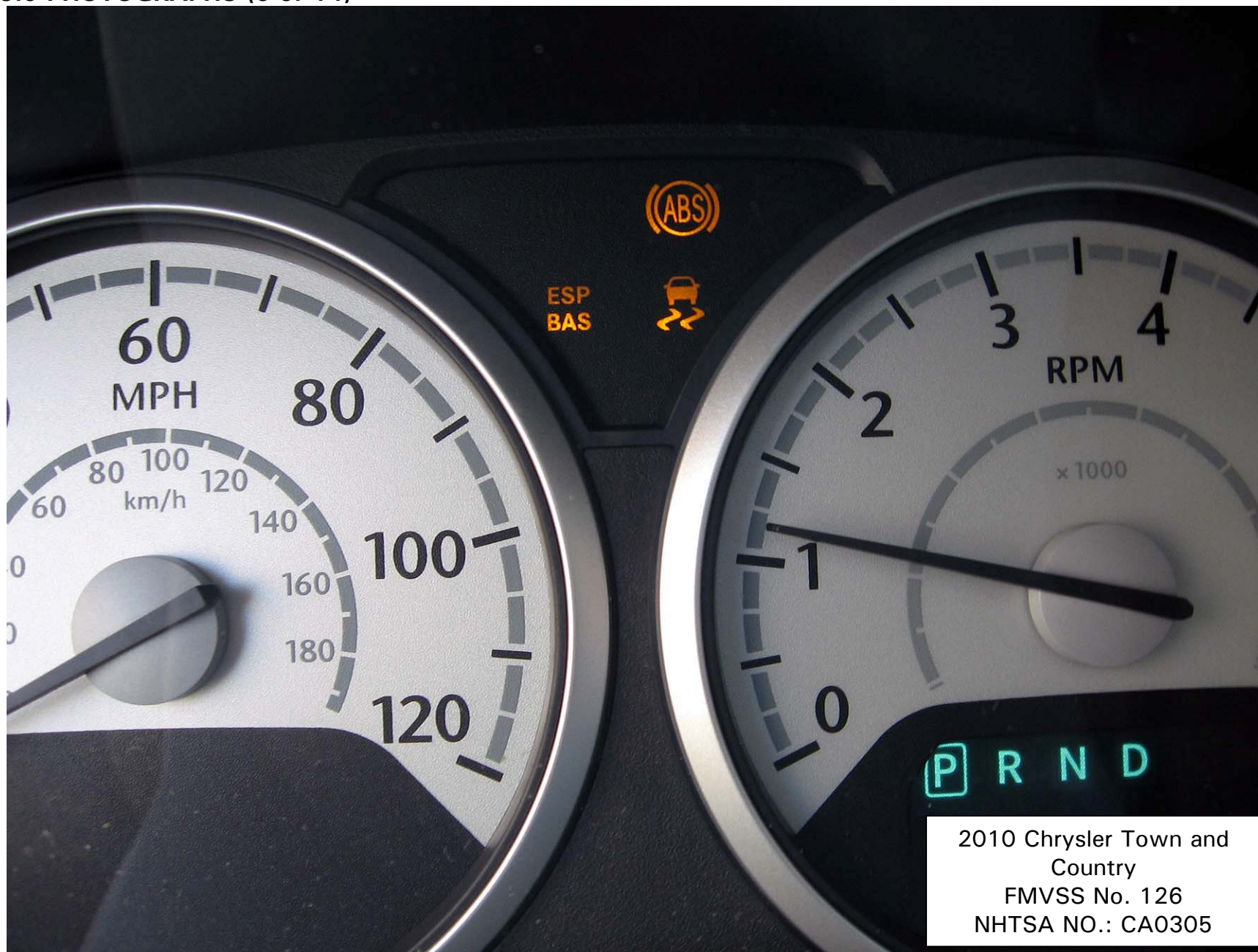
Figure 5.6. Telltale for ESC Malfunction and ESC Off
