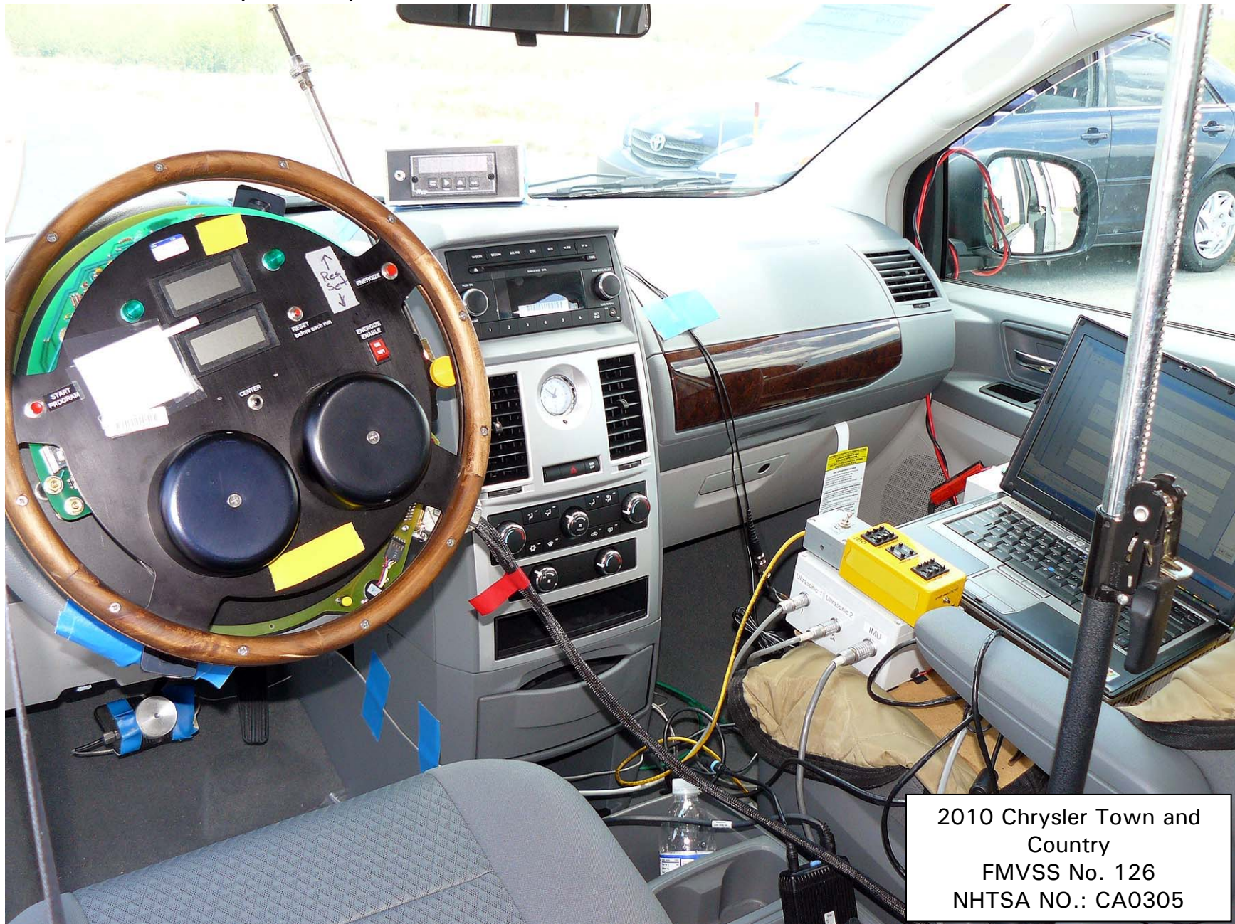
Figure 5.12. Steering Controller and Data Acquisition Computer
