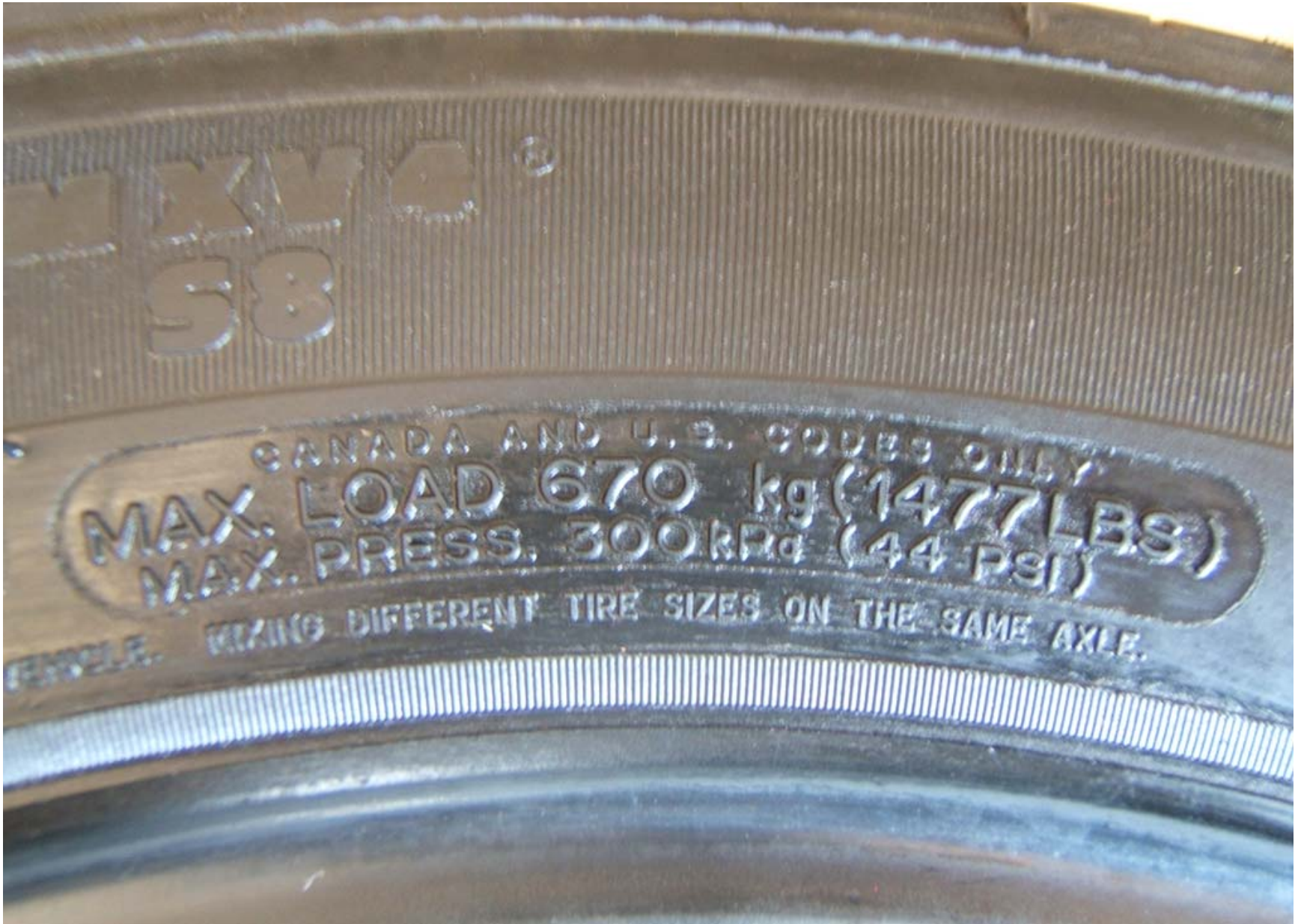
FIGURE 5.9 TIRE SHOWING MAX LOAD RATING AND MAX INFLATION PRESSURE
