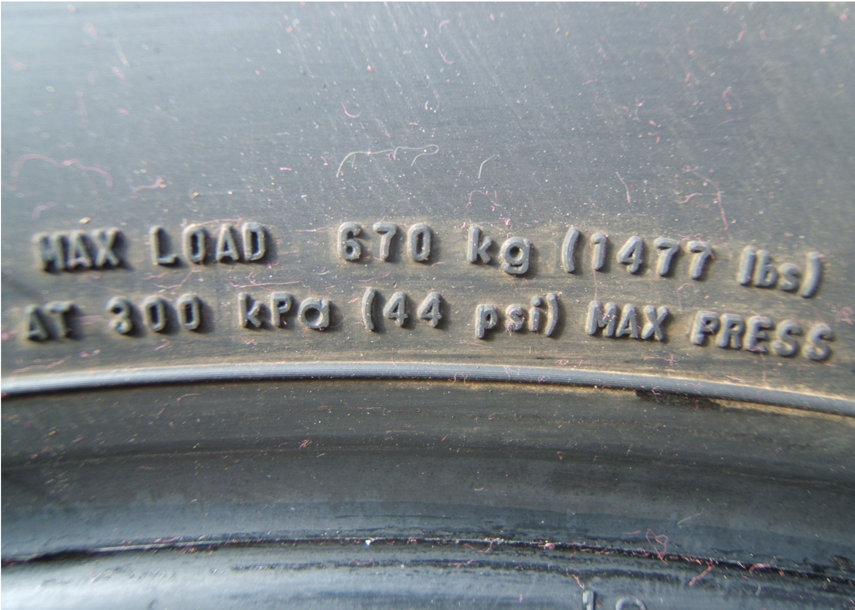
FIGURE 5.7 TIRE SHOWING MAX LOAD RATING AND MAX INFLATION PRESSURE
