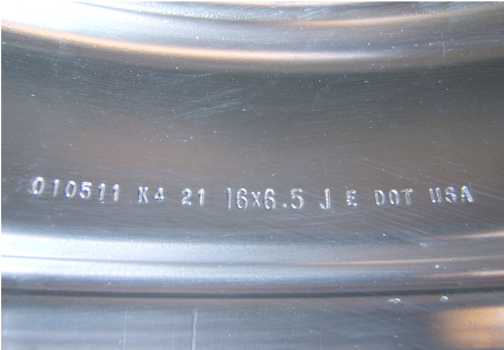
RIGHT FRONT RIM SHOWING DATE OF MANUFACTURE, OTHER RIM MARKINGS, SIZE, LETTER DESIGNATION FOR SOURCE OF PUBLISHED DIMENSIONS, DOT SYMBOL, AND OTHER RIM MARKINGS
