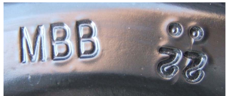
FIGURE 5.11 RIGHT FRONT RIM SHOWING OTHER RIM MARKINGS
