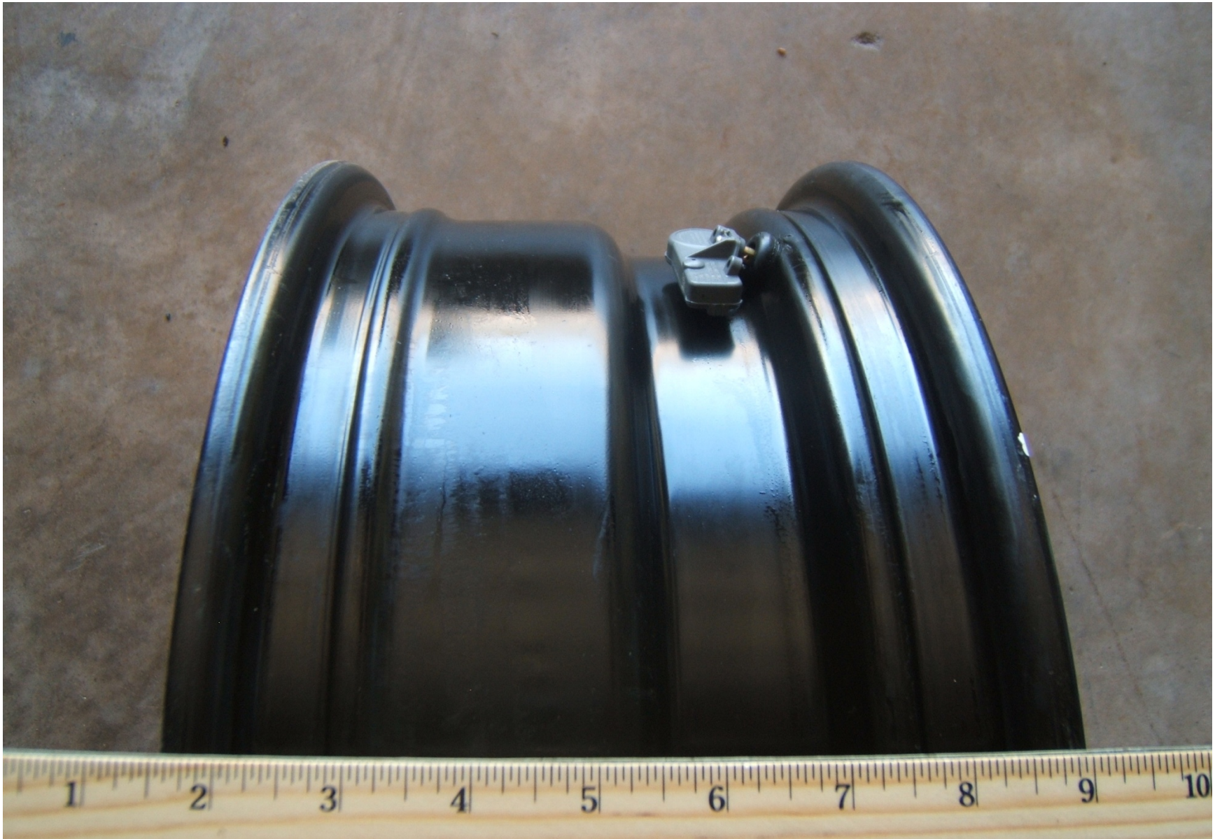
FIGURE 5.9 RIM SHOWING TPMS SENDING UNIT AND RIM CONTOUR FOR FULL WIDTH OF CROSS SECTION
