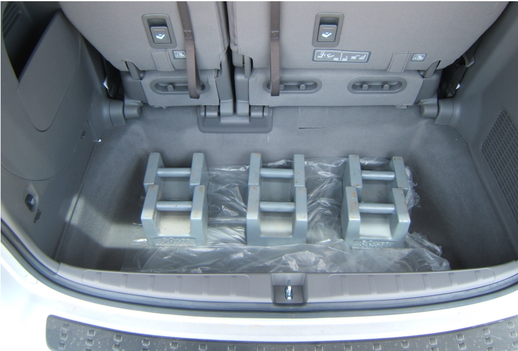
FIGURE 5.17 VEHICLE CARGO AREA BALLAST FOR UVW + VCW LOAD
