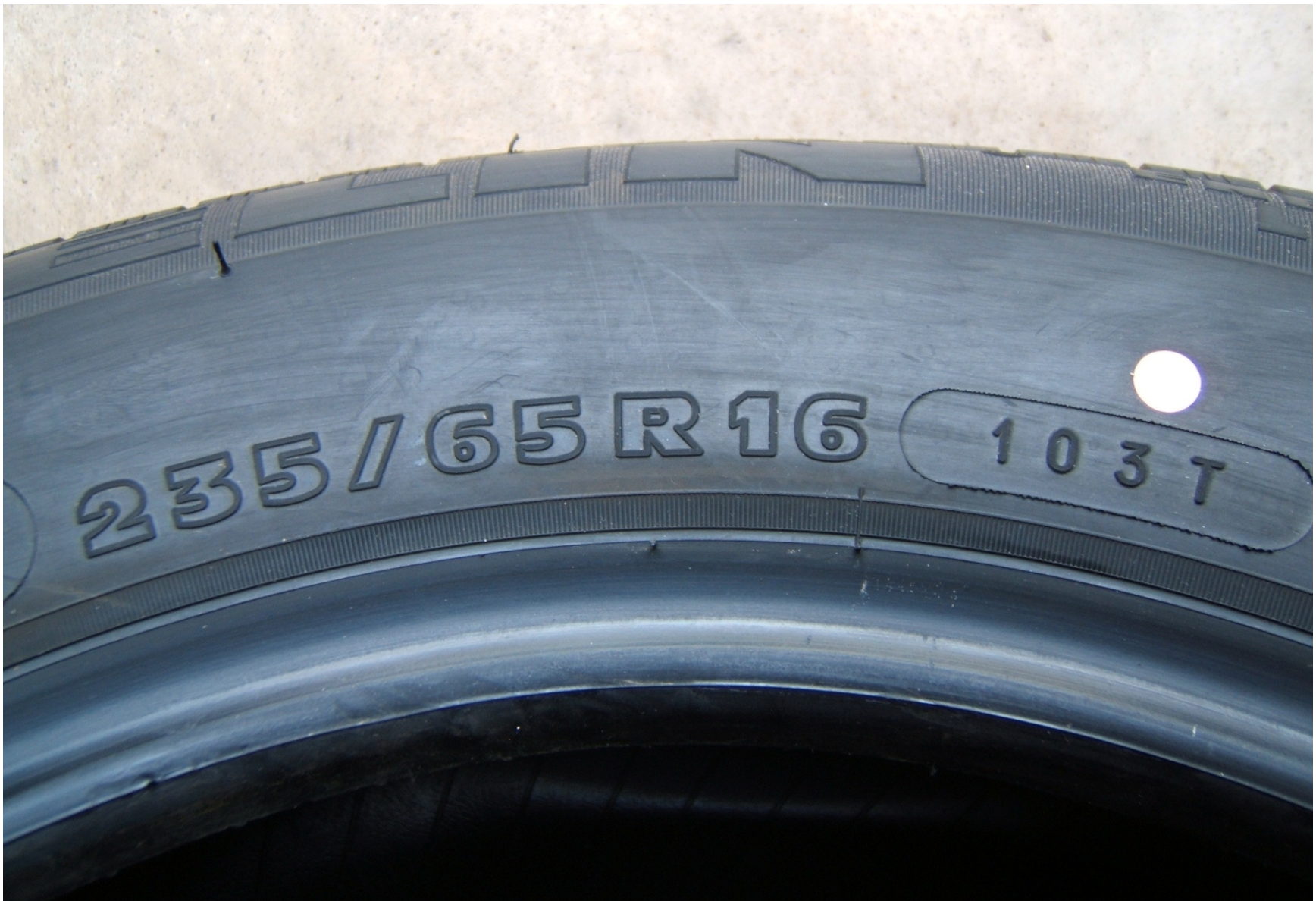
FIGURE 5.6 TIRE SHOWING SIZE AND LOAD INDEX/SPEED RATING
