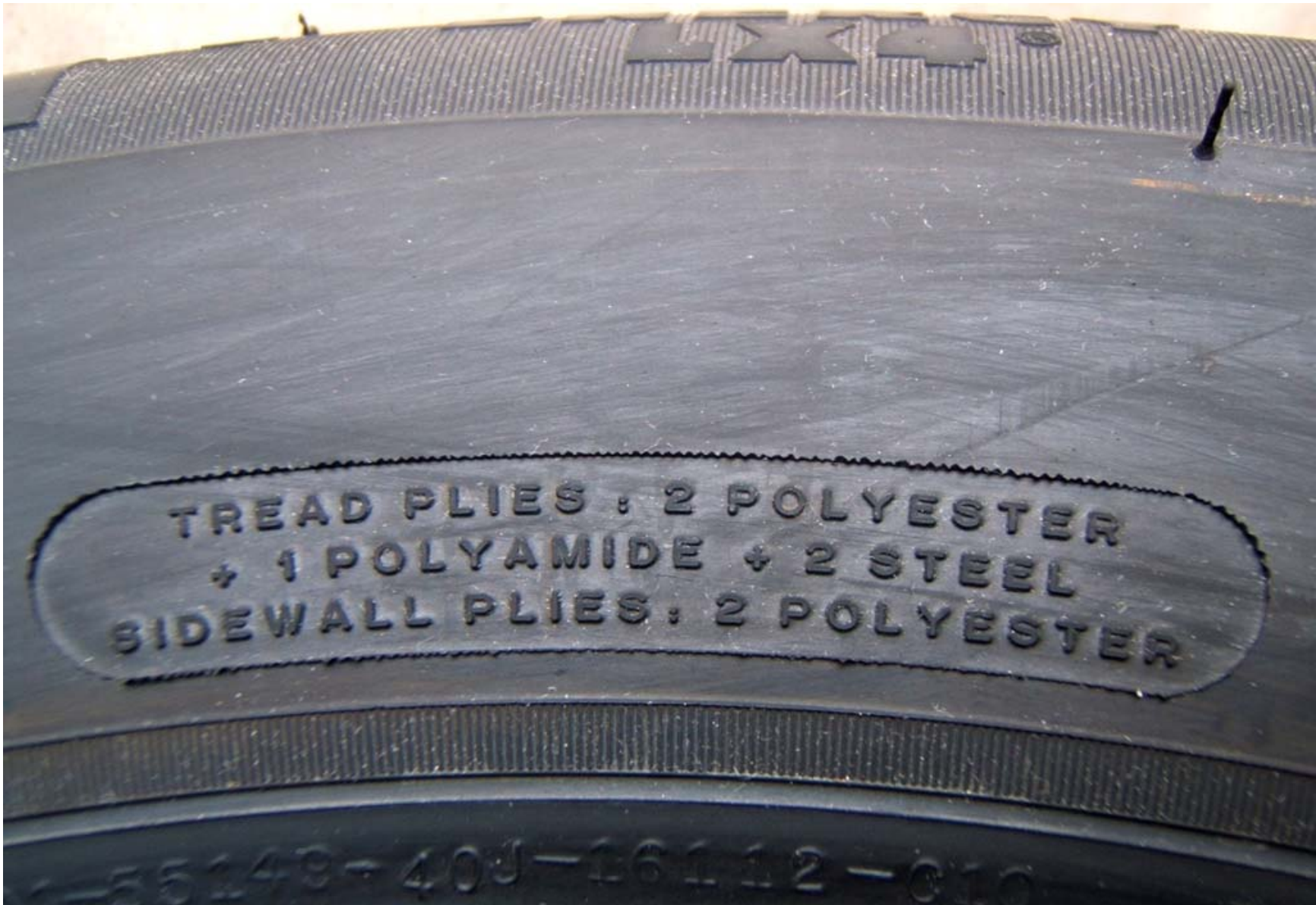
FIGURE 5.9 TIRE SHOWING SIDEWALL / TREAD CONSTRUCTION
