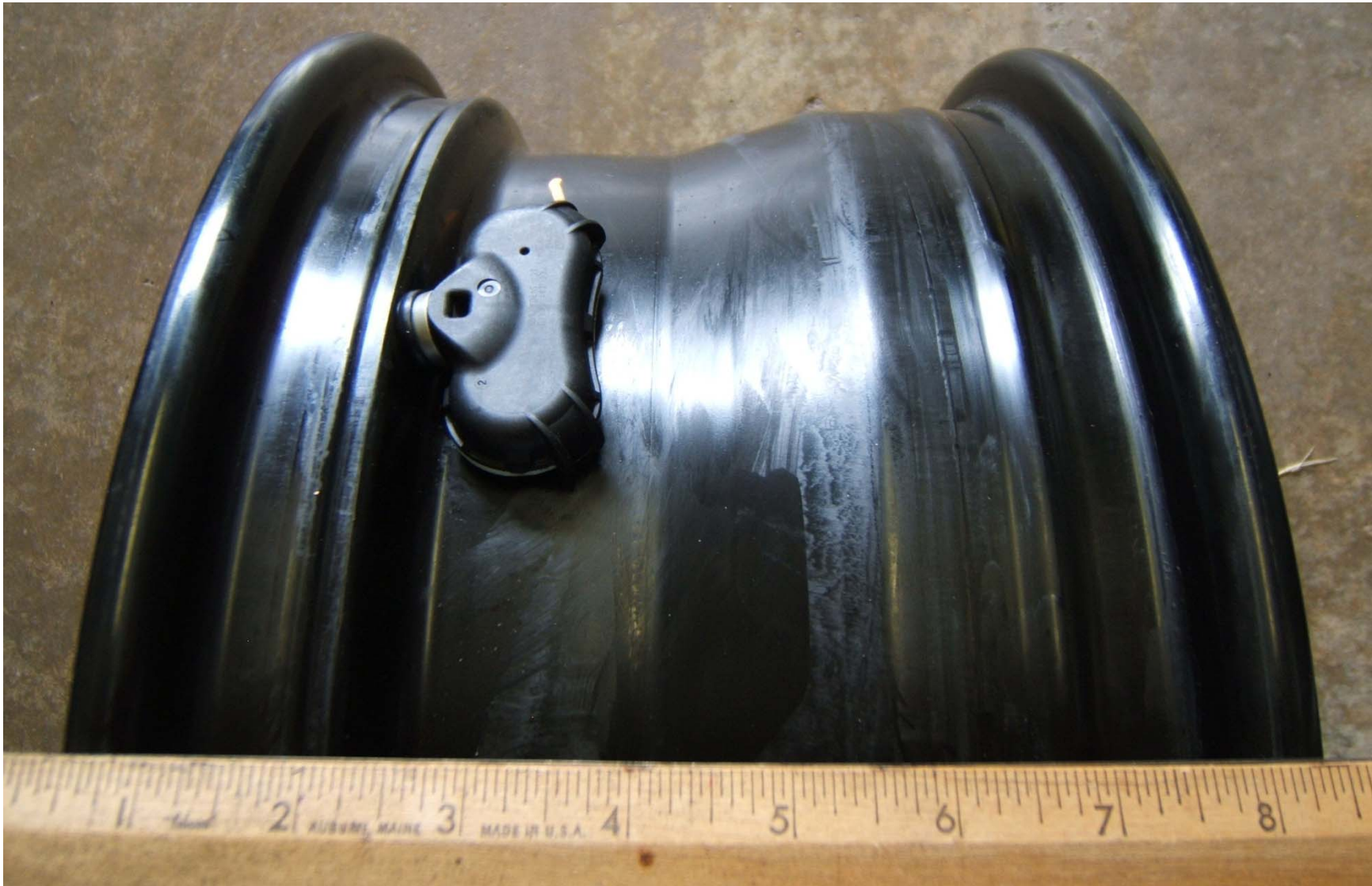
FIGURE 5.10 RIM SHOWING TPMS SENSOR AND RIM CONTOUR FOR FULL WIDTH OF CROSS SECTION
