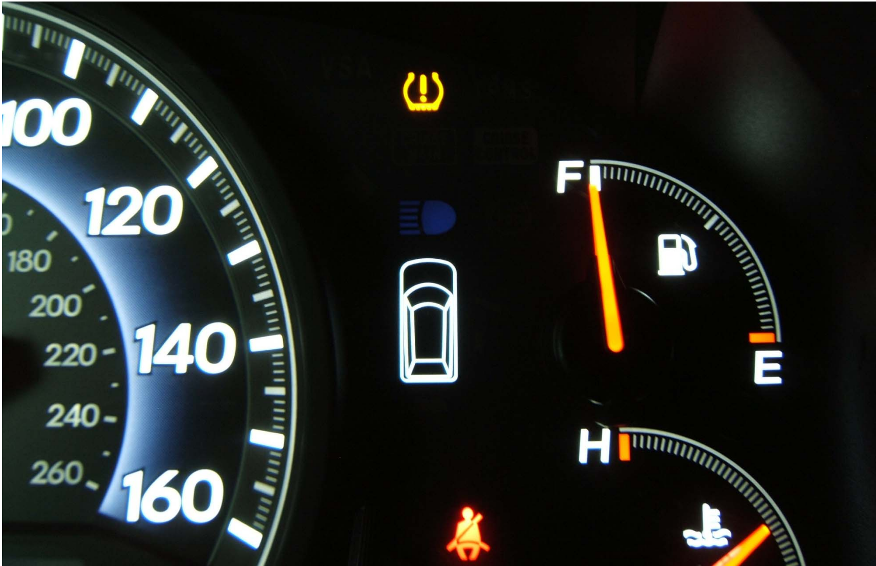
FIGURE 5.11 DISPLAY SHOWING LOW TIRE PRESSURE WARNING TELLTALE
