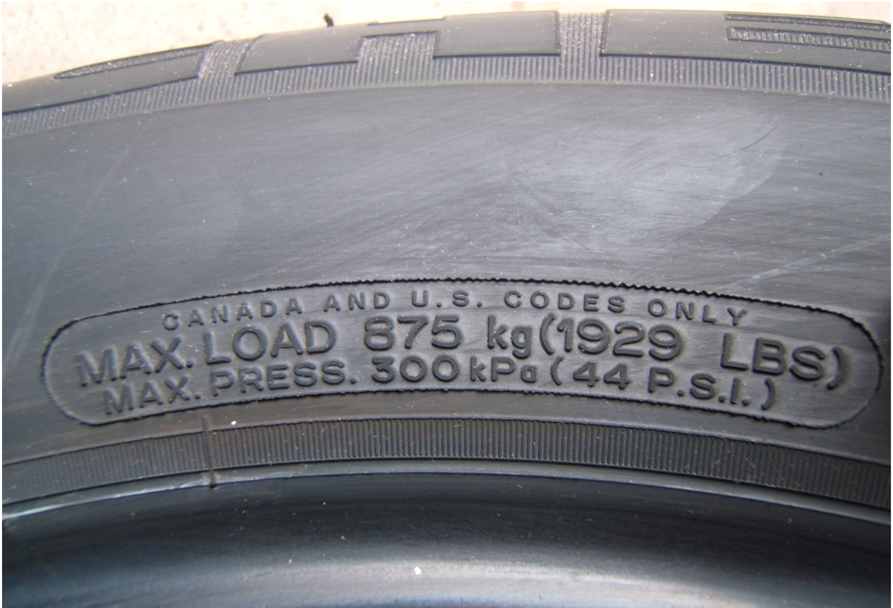
FIGURE 5.8 TIRE SHOWING MAX LOAD RATING AND MAX COLD INFLATION PRESSURE
