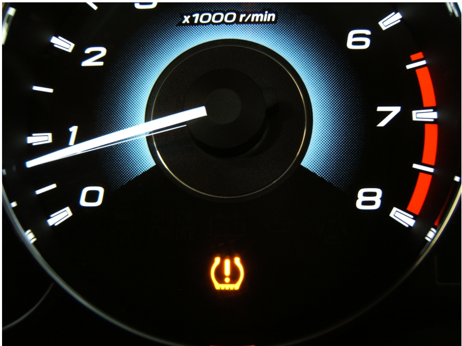
FIGURE 5.11 DISPLAY SHOWING COMBINATION LOW TIRE PRESSURE / TPMS MALFUNCTION WARNING TELLTALE
