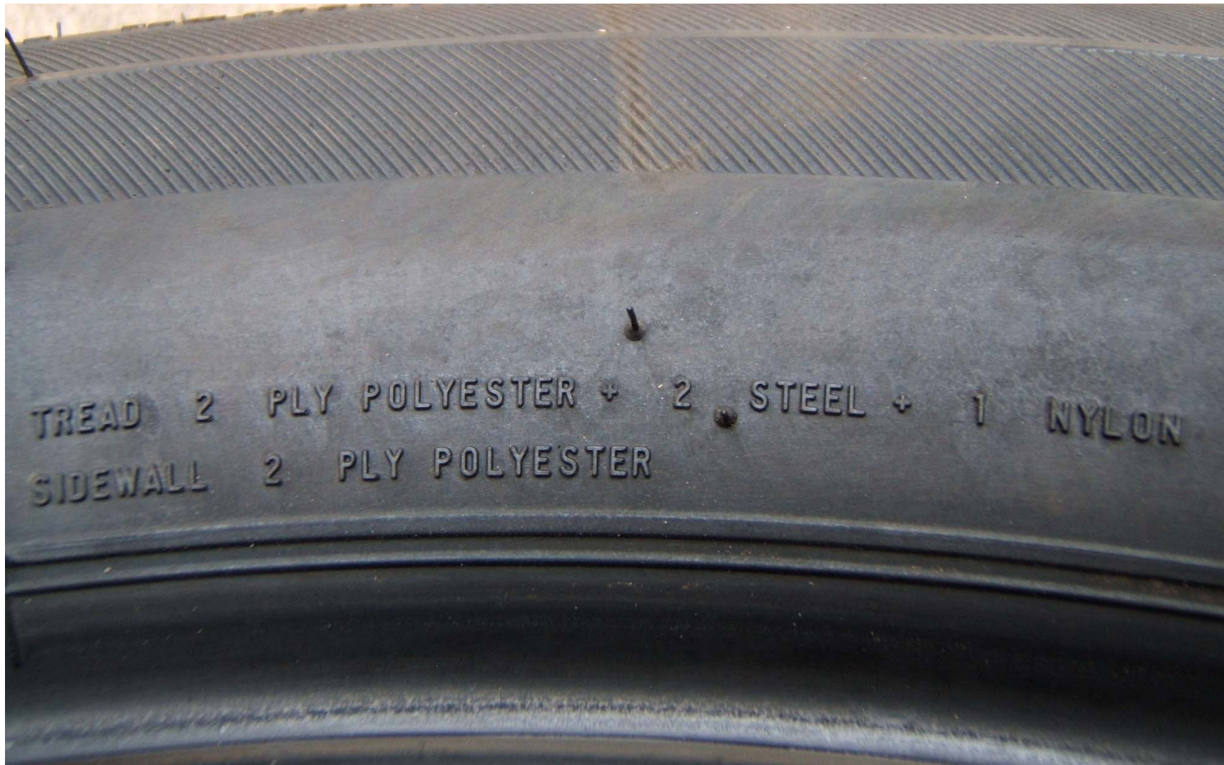
FIGURE 5.9 TIRE SHOWING SIDEWALL / TREAD CONSTRUCTION
