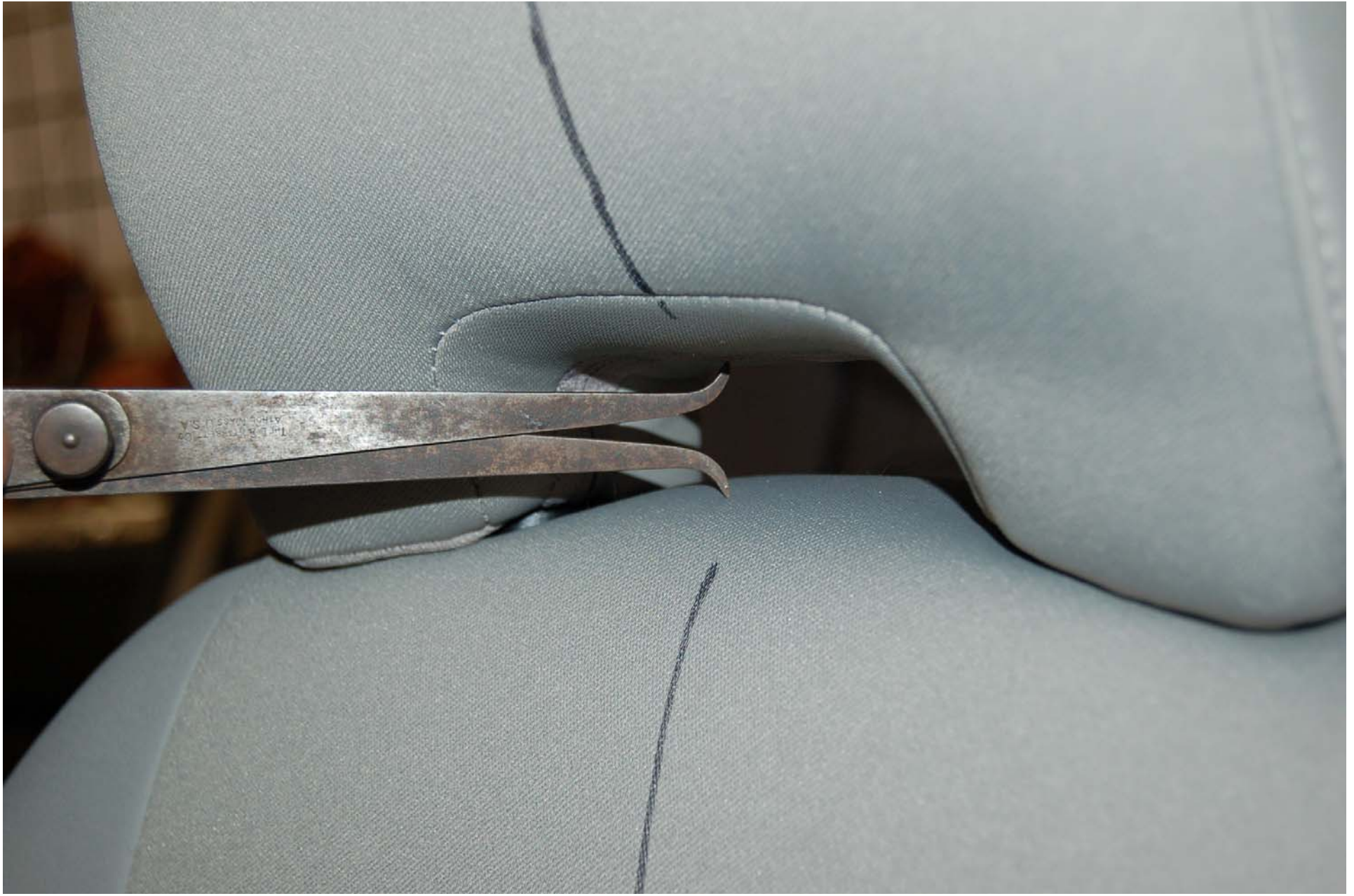
FIGURE 5.12 FRONT HEAD RESTRAINT GAP MEASUREMENT
