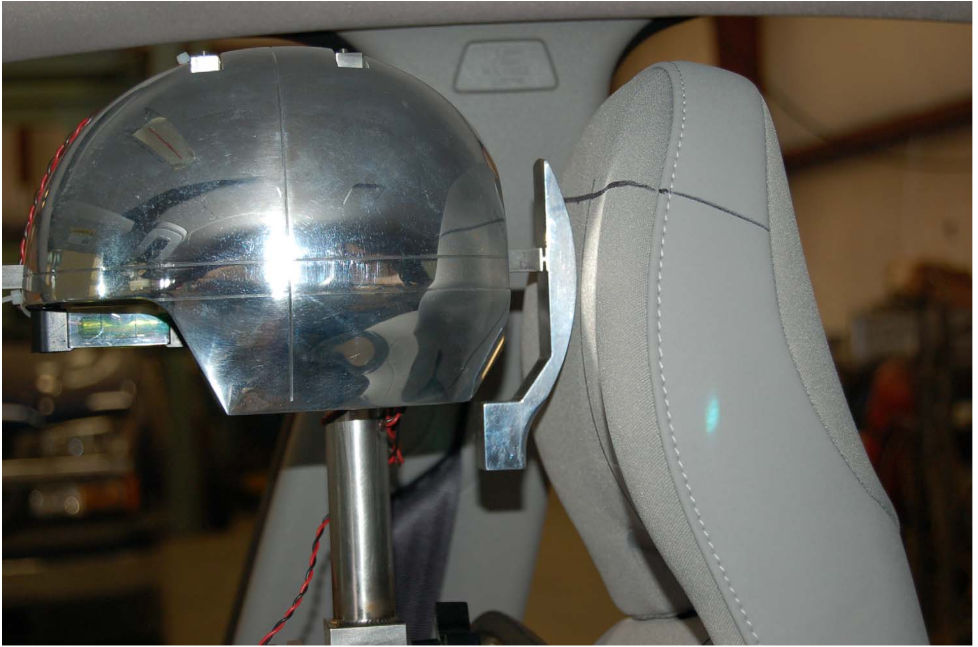
FIGURE 5.26 MEASUREMENT OF FRONT PASSENGER SEAT BACKSET
