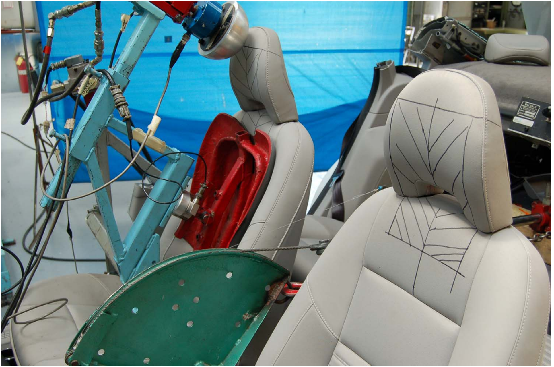
FIGURE 5.35 BACK PAN LOADED TO 373 Nm
