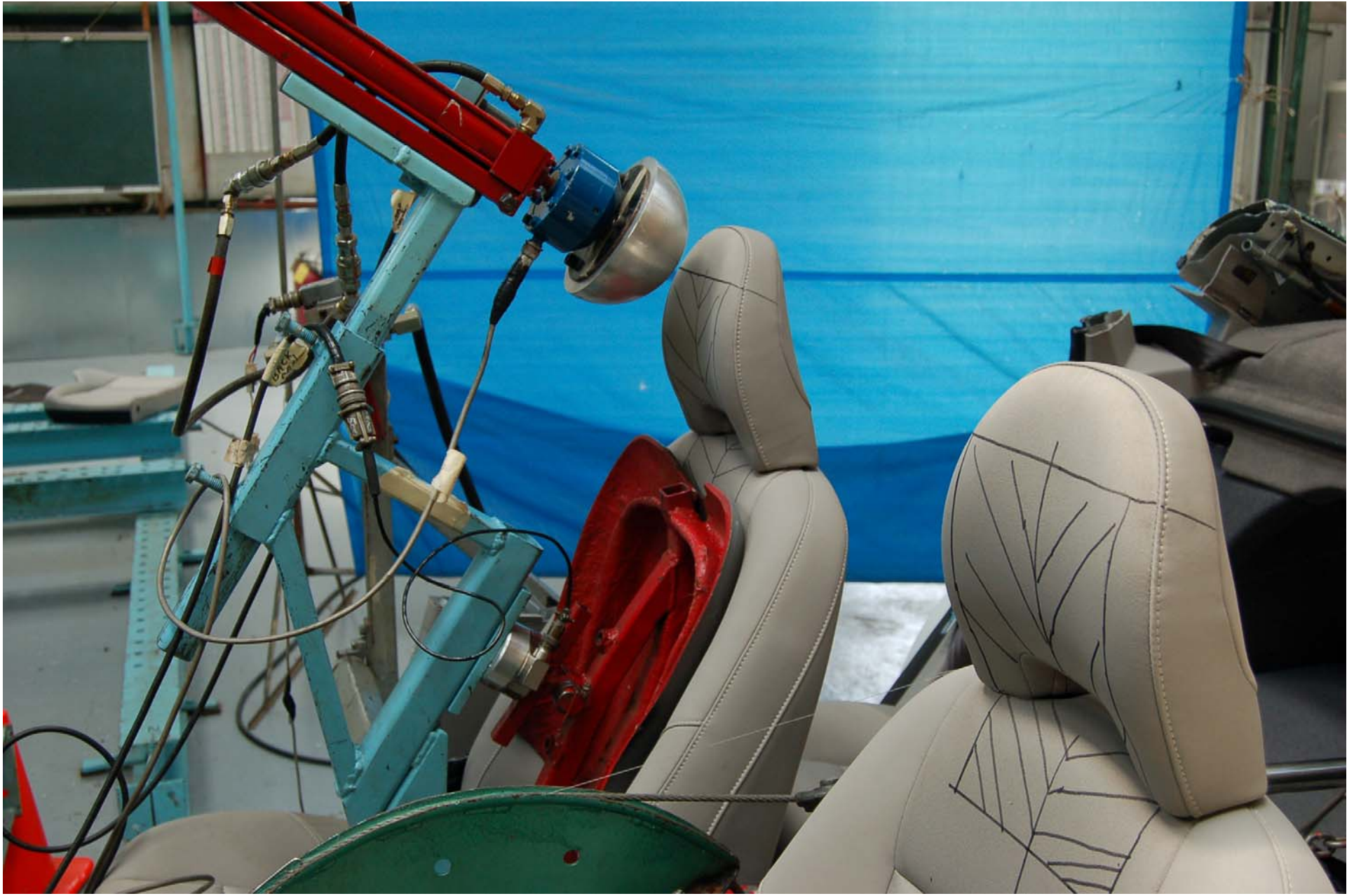
FIGURE 5.40 HEAD RESTRAINT POST TEST
