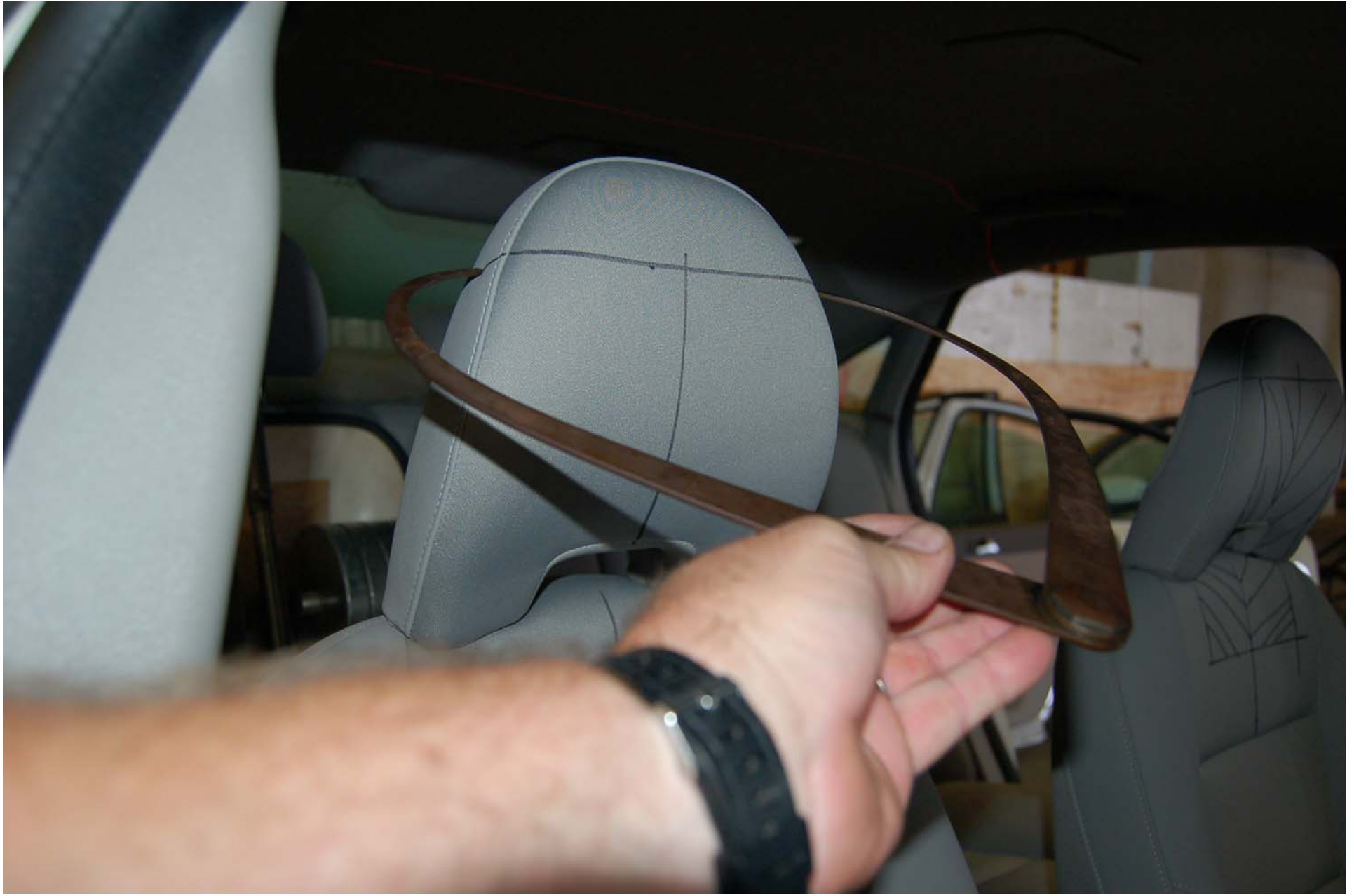
FIGURE 5.18 WIDTH MEASUREMENT ON FRONT PASSENGER SEAT HEAD RESTRAINT
