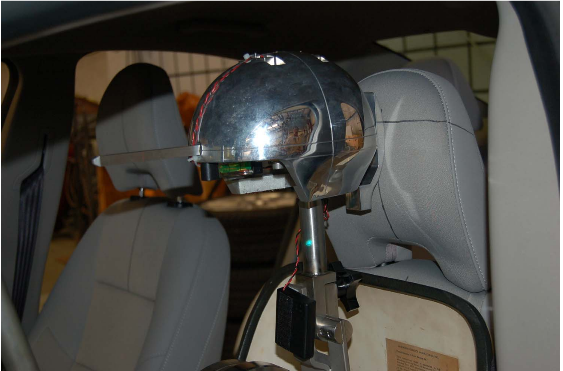
FIGURE 5.22 HRMD IN FRONT DRIVER SEAT
