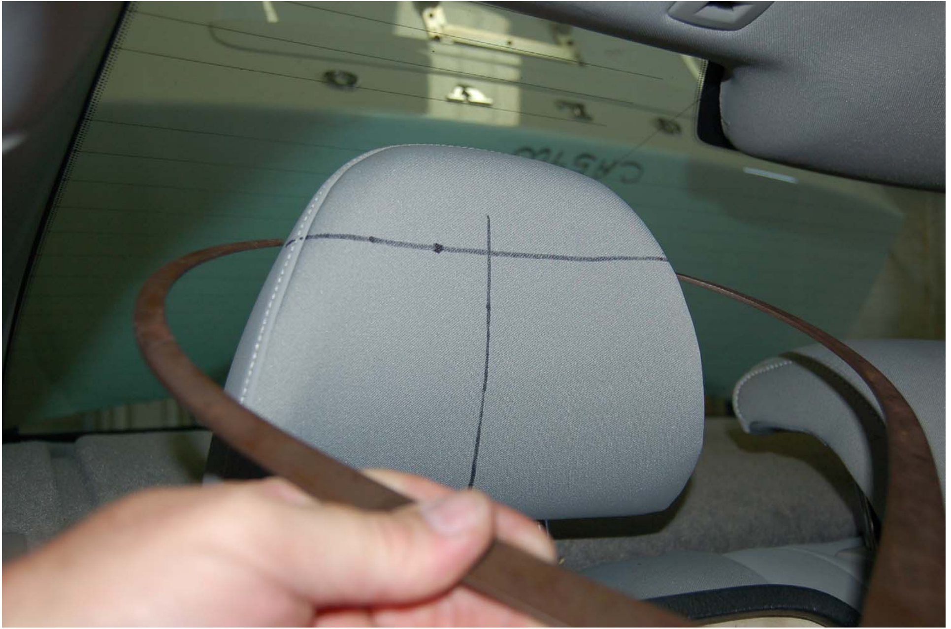
FIGURE 5.20 WIDTH MEASUREMENT OF REAR PASSENGER SEAT HEAD RESTRAINT
