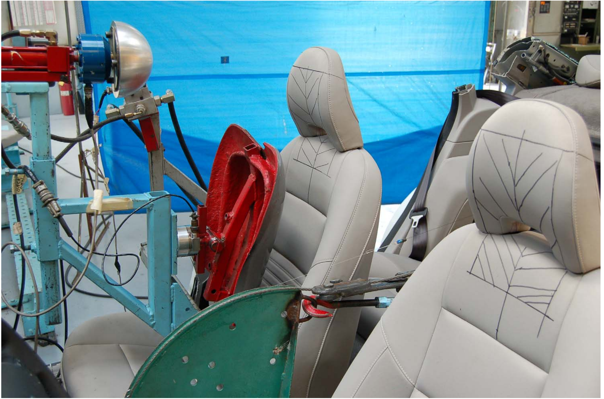
FIGURE 5.34 PRE-TEST SET-UP FOR BACKSET RETENTION
