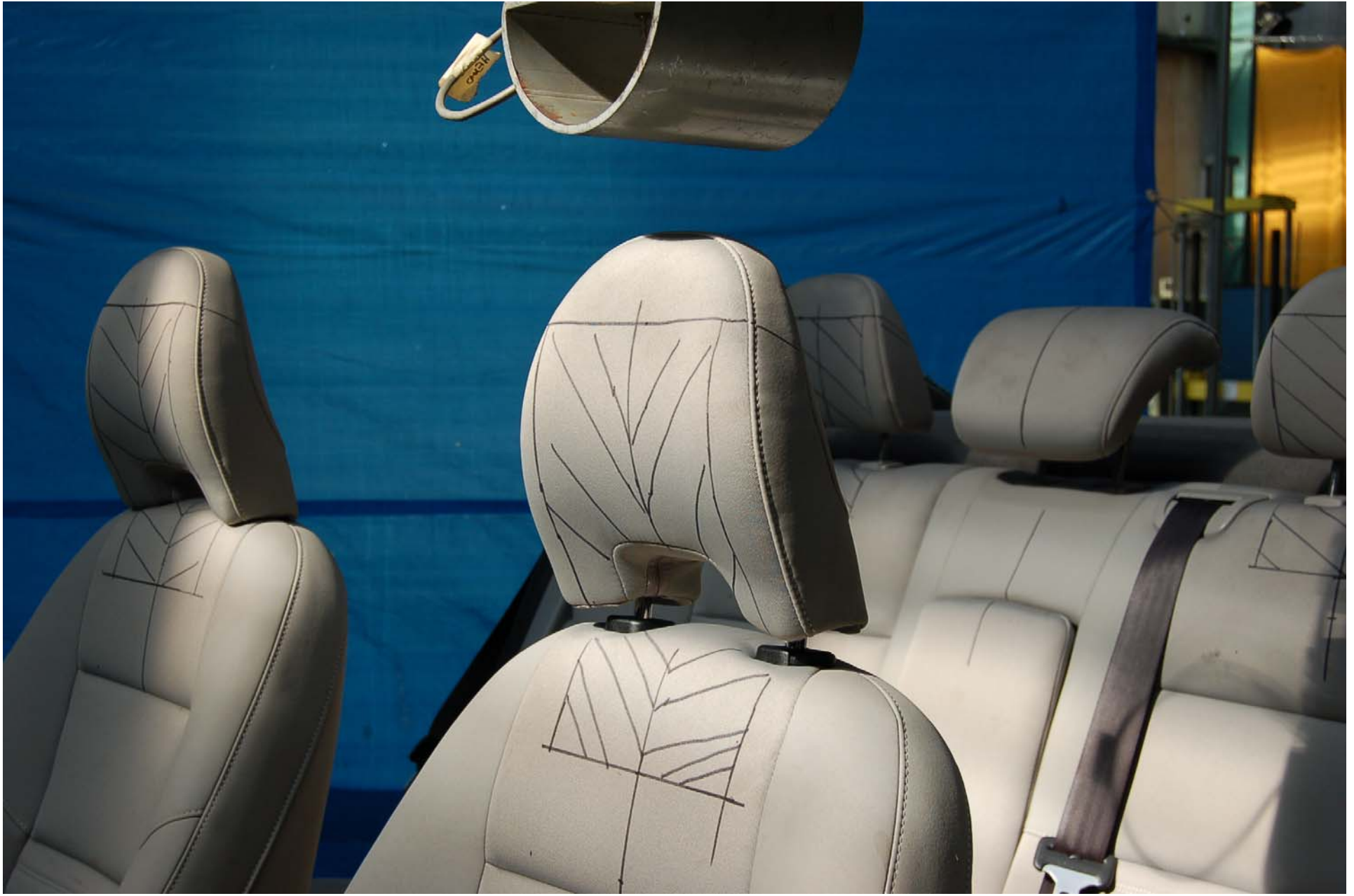
FIGURE 5.33 HEAD RESTRAINT POST TEST HEIGHT RETENTION
