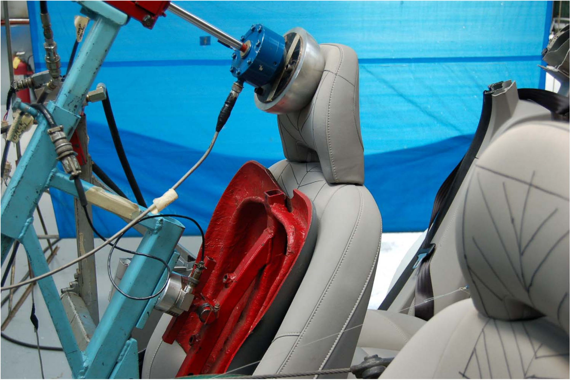
FIGURE 5.39 HEAD FORM AT 895 N LOAD
