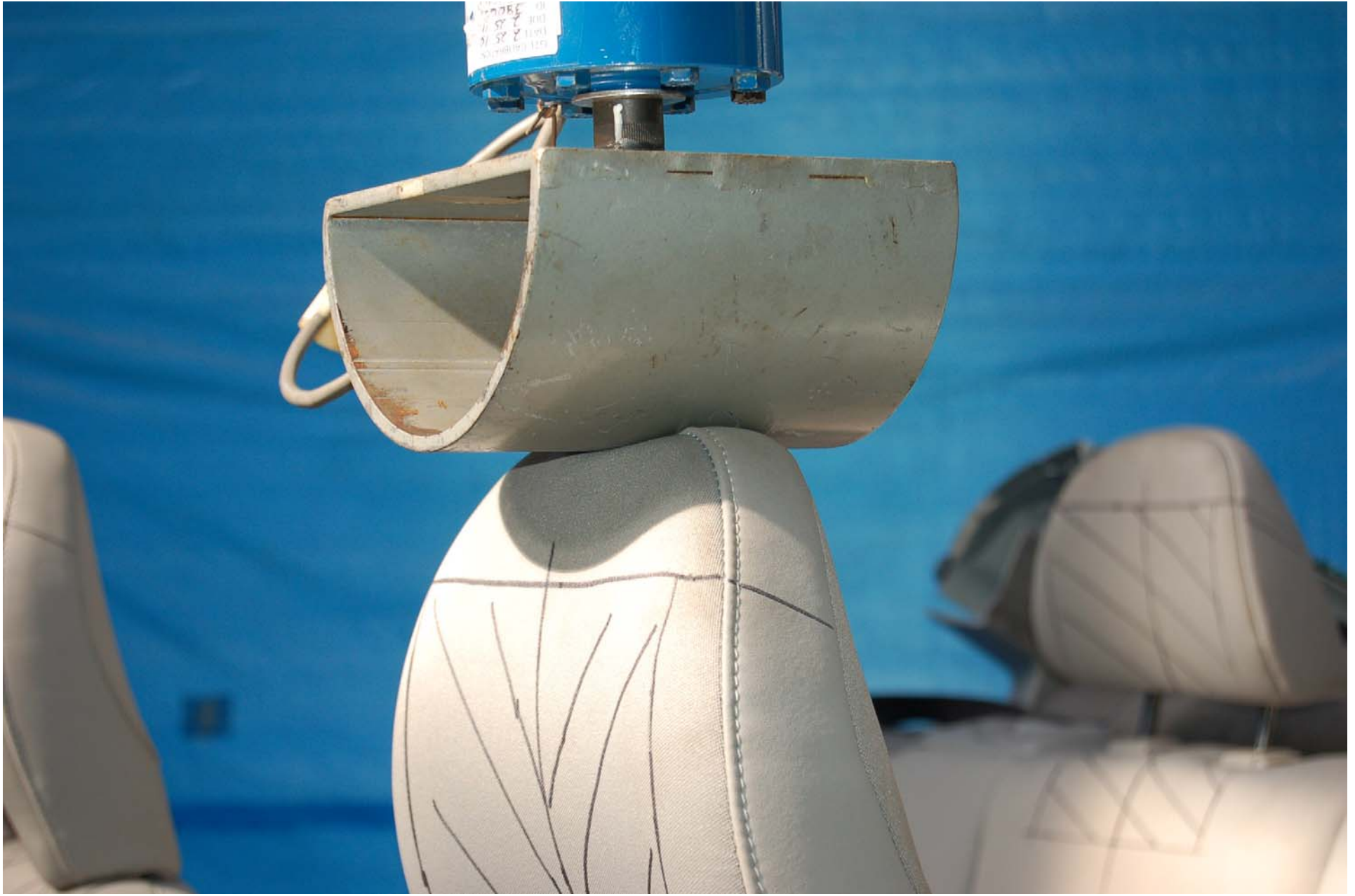
FIGURE 5.31 HEAD RESTRAINT AT FULL LOAD
