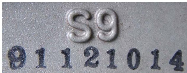
FIGURE 5.10 RIM MARKINGS INCLUDING LETTER DESIGNATION FOR SOURCE OF PUBLISHED DIMENSIONS, DOT SYMBOL, MANUFACTURER SYMBOL, RIM SIZE, AND MANUFACTURE DATE
